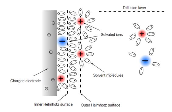
Fig. 3 Diagram of the Helmholtz double layer on a liquid-solid (electrolyte-electrode) interface.
