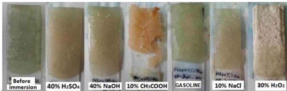
**Figure 13.** Samples of epoxy composites composed of the waste glass (WGS) and the ER1 polymeric matrix after 28 days of exposure to various chemically aggressive environments.
