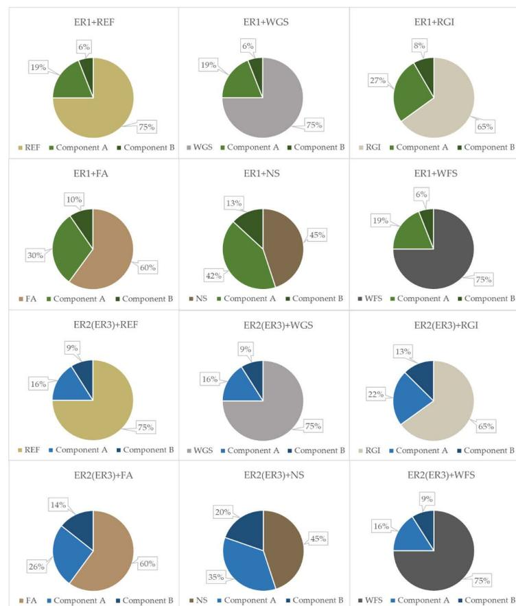
**Figure 2.** Tested formulations of the epoxy composites (ER—Epoxy resin, REF—Reference filler, WGS—Waste glass from solar panels, RGI—Waste from the production of mineral insulation boards, FA—Fly ash, NS—Neutralisation sludge, WFS—Waste foundry sand).
