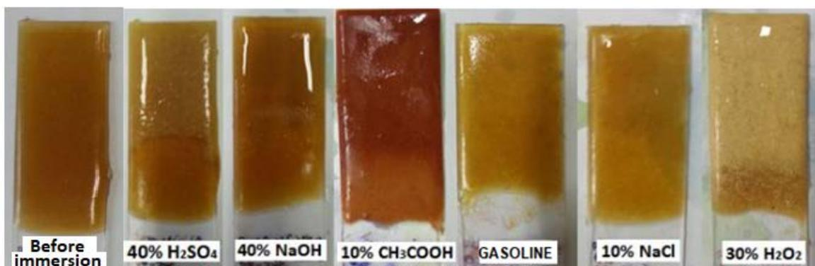
**Figure 15.** Samples of epoxy composites composed of the RGI filler and the ER3 polymeric matrix after 28 days of exposure to various chemically aggressive environments.
