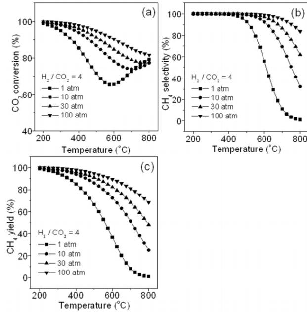
Fig. 4-1: Effects of pressure and temperature with  $\text{H}_2/\text{CO}_2 = 4$  on  $\text{CO}_2$  methanation: (a)  $\text{CO}_2$  conversion, (b)  $\text{CH}_4$  selectivity, and (c)  $\text{CH}_4$  yield [30]
