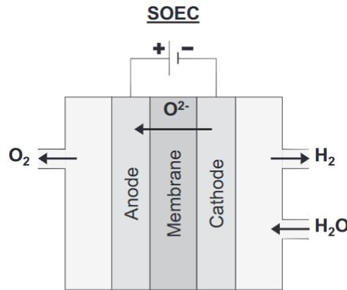
Fig. 2-3: Solid oxide electrolysis [15]
