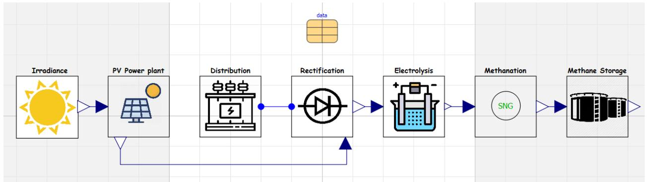
Fig. 6-1: Overall power-to-gas model
