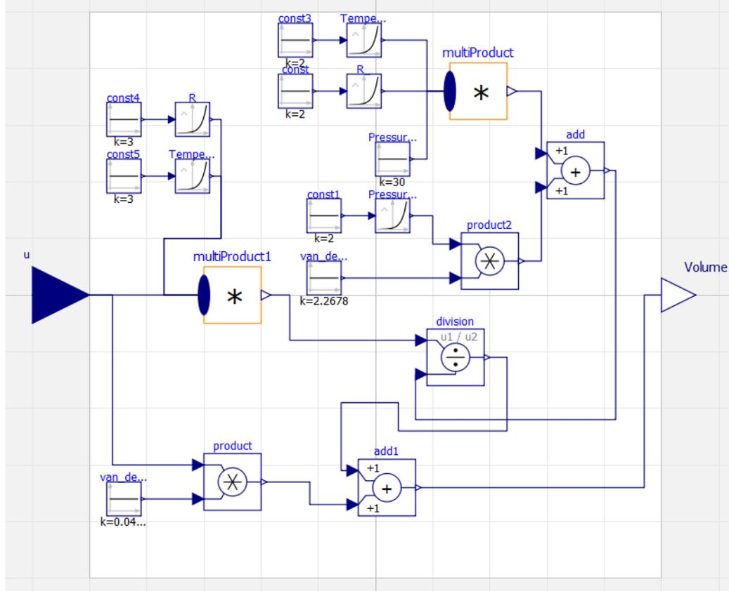
Fig. 6-8: Van der Waals equation model
