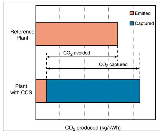
Fig. 3-6:  $CO_2$  emission intensity with and without carbon capture [24]
