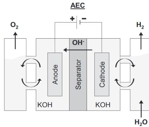
Fig. 2-1: Alkaline electrolysis [15]
