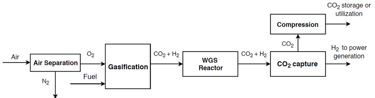
Fig. 3-3: Pre-combustion capture [21]
