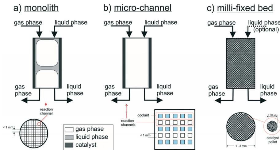
Fig. 4-7: Structured micro-reactors [35]
