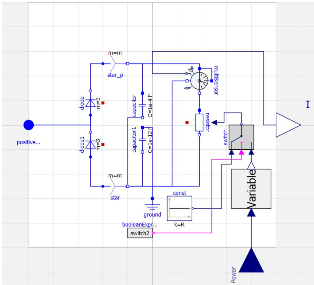
Fig. 6-6: Rectification model
