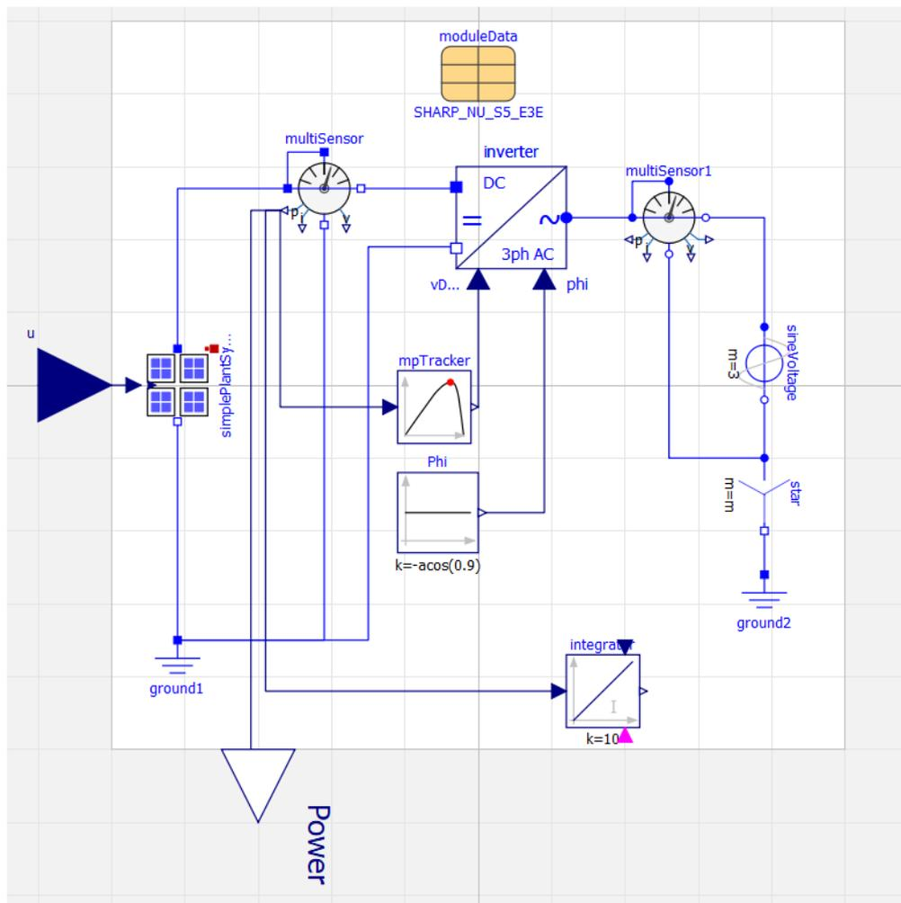
Fig. 6-3: PV power plant model
