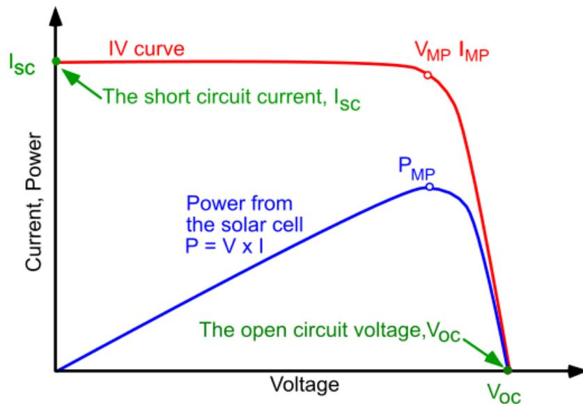
Fig. 6-4: IV curve of a solar cell [39]
