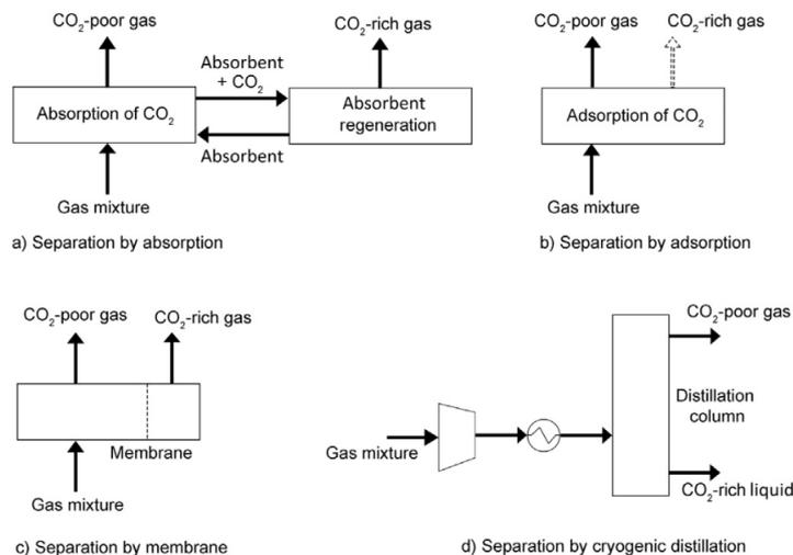
Fig. 3-5:  $\text{CO}_2$  separation technologies [22]
