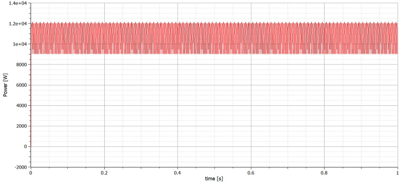
*Fig. 6-15: Active power from 22 kV MV network*
