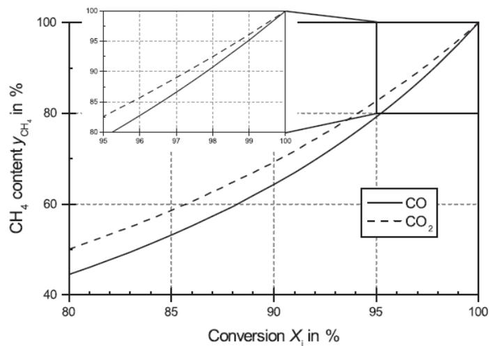
Fig. 4-2:  $\text{CH}_4$  content at different  $\text{CO}_2$  conversion rates [7]
