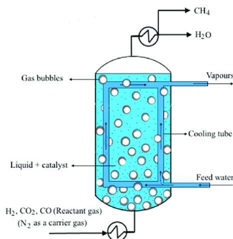
Fig. 4-6: Three-phase reactor [34]
