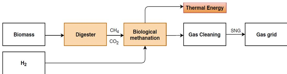
Fig. 4-8: Biological methanation in a separate reactor [7]
