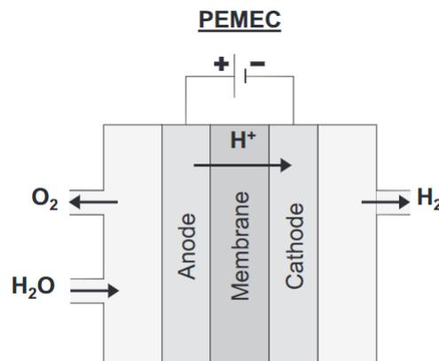
Fig. 2-2: Polymer electrolyte membrane electrolysis [15]
