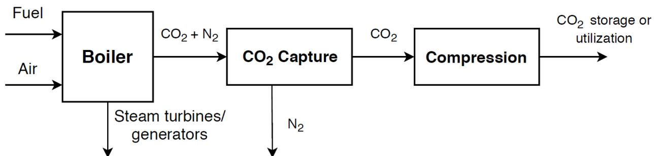
Fig. 3-2: Post-combustion capture [21]
