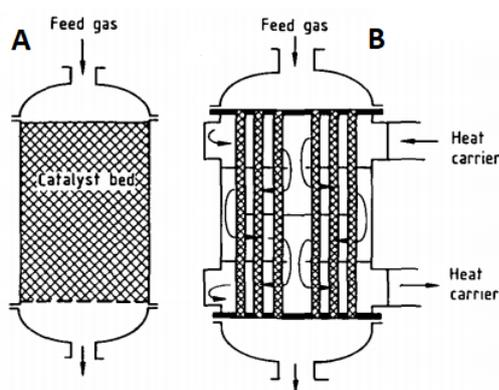
*Fig. 4-4: Catalytic fixed-bed reactors A) Adiabatic fixed-bed reactor; B) Multi-tubular fixed-bed reactor [32]*
