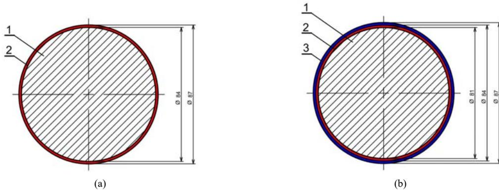
Fig. 2. Cylindric specimens for experimental campaign made of a steel substrate (numbered as 1) and (a) one thin laser-cladded layer (numbered as 2); (b) two thin laser-cladded layers (numbered as 3).
