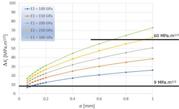
Fig. 6. Dependence of the stress intensity factor range on the crack length for various Young's moduli of the cladded layer with the thickness  $h_1 = 2$  mm.
