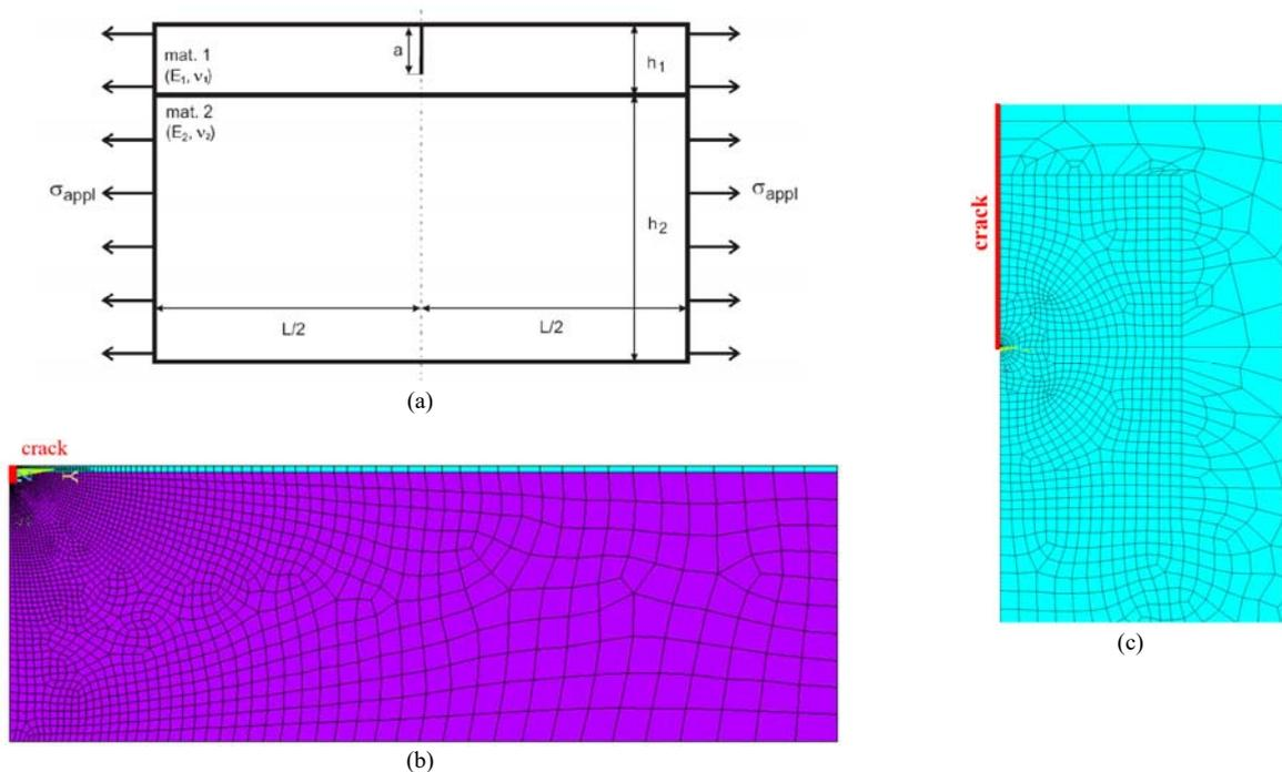
Fig. 4. Simplified numerical model: (a) schema and dimensions; (b) FE mesh of the right half of the specimen with the crack in the upper left corner; (c) detail of the refined FE mesh around the crack tip.
