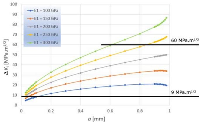
Fig. 5. Dependence of the stress intensity factor range on the crack length for various Young's moduli of the cladded layer with the thickness  $h_1 = 1$  mm.
