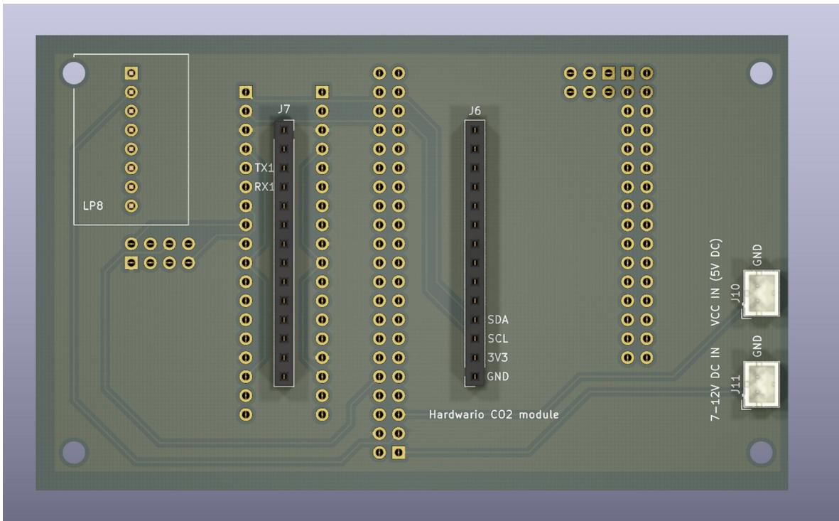
Figure 4.20: Render of the alternative PCB with JST connectors.
