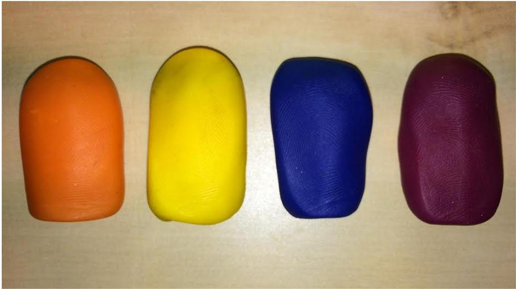
Figure 7.4: Various fake fingers from Fimo material.
