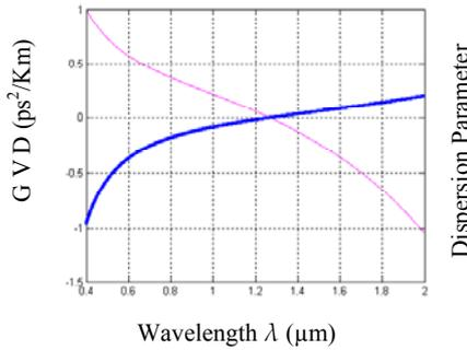
Fig. 3. Variation of group velocity dispersion  $k''$  and dispersion parameter  $D$  (solid line) with wavelength for fused silica.
