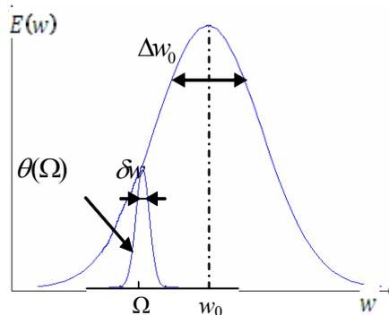
**Fig. 6.** Gaussian envelope decomposed into a number of wavelets.
