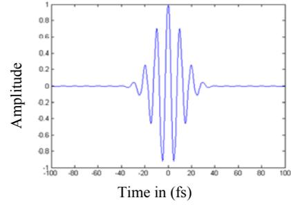
Fig. 1. The electric field of an ultra-short lasers pulse consisting of only a few cycles.
