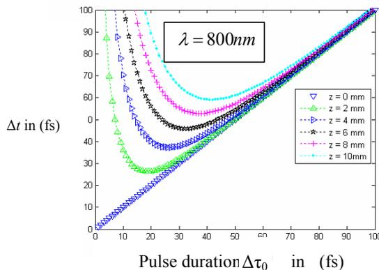
Fig. 4. Temporal broadening of the transform-limited pulse for different values of the propagation distance  $z$ .
