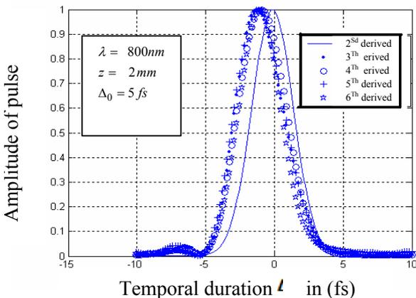
**Fig. 5.b** The pulse shape is no longer Gaussian and it becomes asymmetric due to higher order dispersion.
