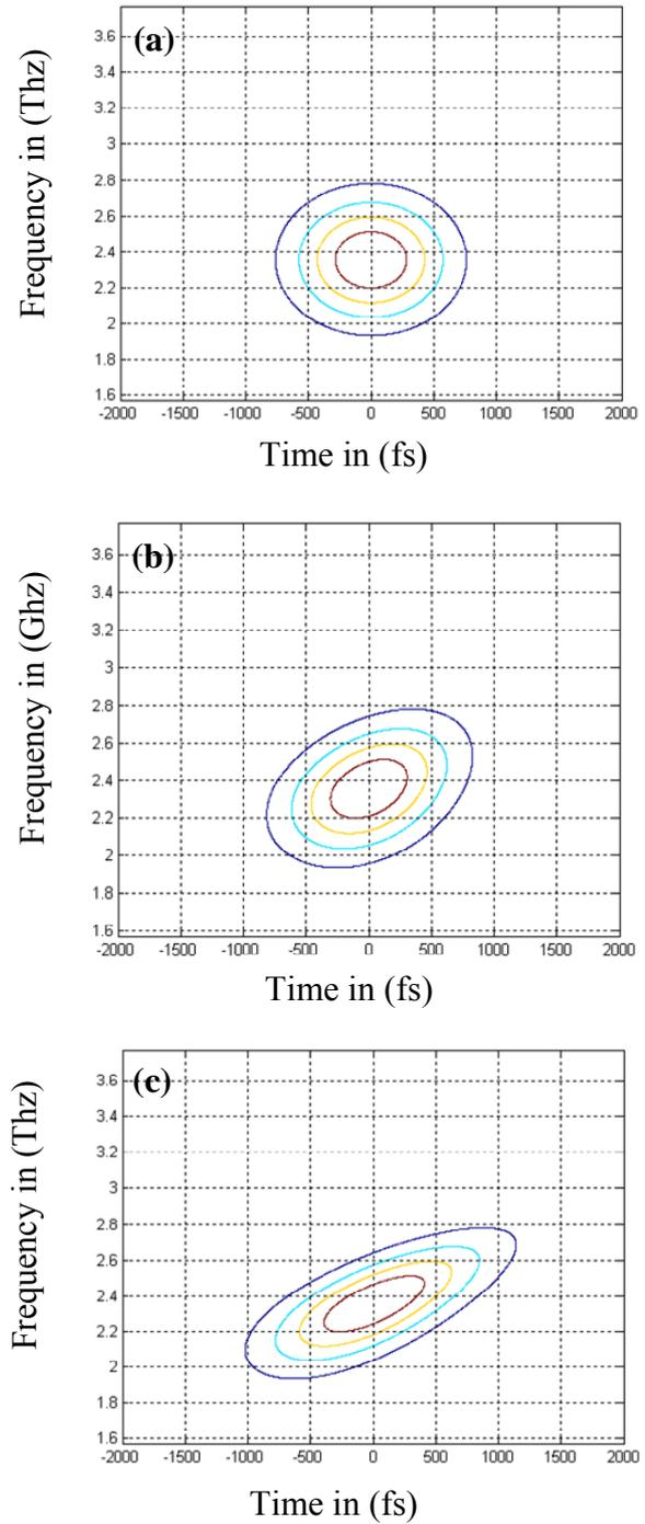
**Fig. 8.** (a) Contour of the initial wavelet, (b) contour of the wavelet after propagation of 2 cm in the fused silica, (c) contour of the wavelet after propagation of 5cm in the fused silica.
