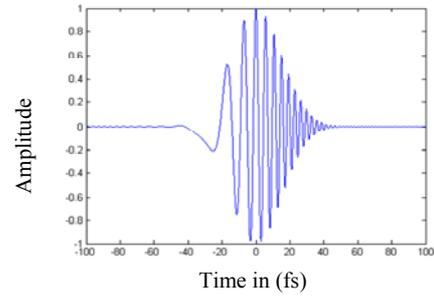
Fig. 2. The electric field of an ultrashort lasers pulse with a strong positive chirp. Note the frequency variation as a function of time; at the leading edge (to the left) the wavelength is longer than at the trailing edge.
