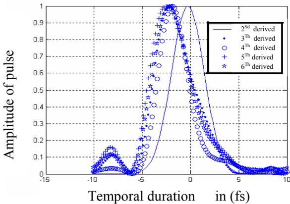
**Fig. 5.a** The pulse broadens on propagation as a result of group velocity dispersion (GVD) ( $\lambda=800$  nm,  $z=4$  mm).
