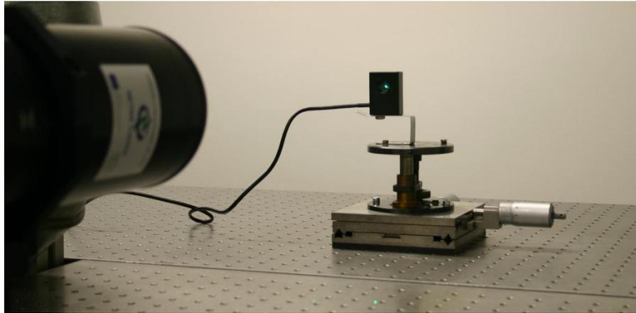
Figure 6-5 Setting up beams with PDA camera.
