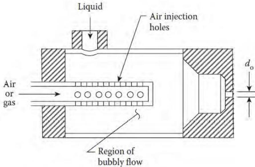
Figure 1-4 Schematic layout of effervescent atomizer. [1]
