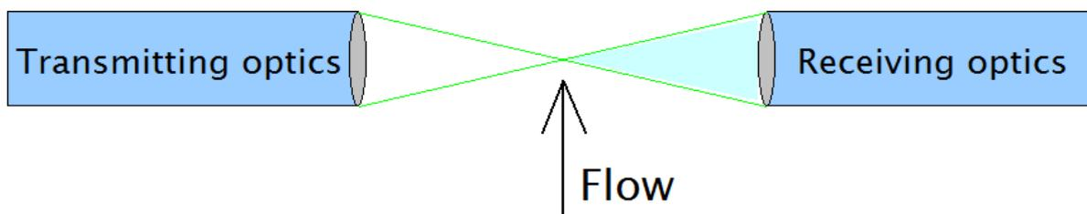
Figure 4-6 Forward scattering LDA.
