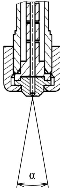
Figure 7-4 Spray Cone angle.
