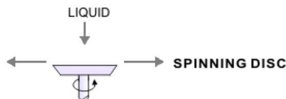
Figure 1-2 Rotary atomizer. [4]
