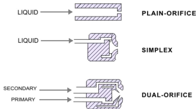
Figure 1-1 Pressure nozzles. [4]
