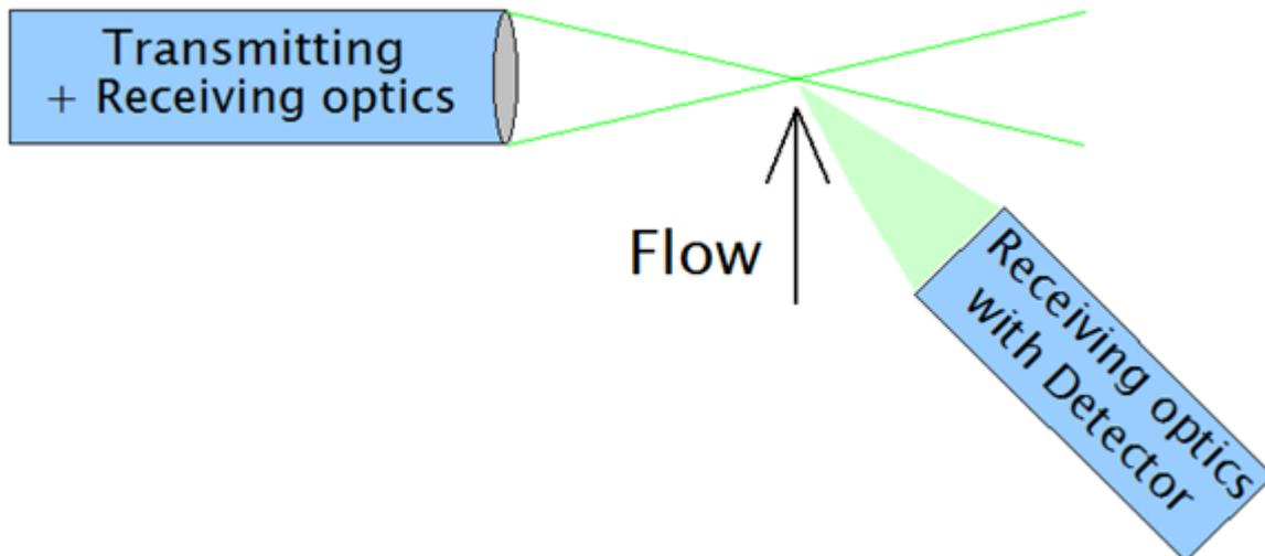
Figure 4-9 Off-axis scattering LDA.
