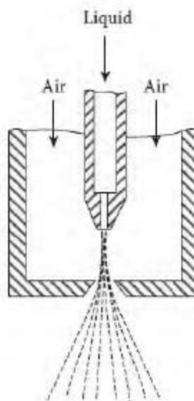
Figure 1-5 Air-blast atomizer. [4]
