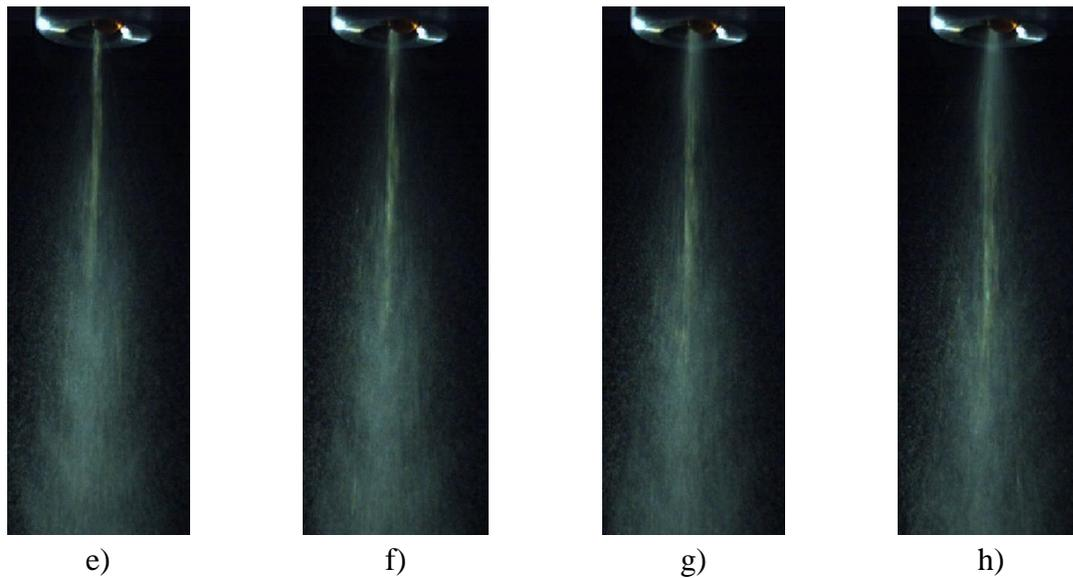
Figure 7-3 Instability in spray (GLR = 2%,  $p = 2\text{bar}$ ).
