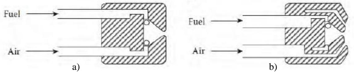
Figure 1-3 Construction of air-assist atomizers: a) internal mixing b) external mixing. [1]
