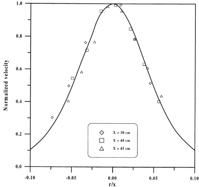
Figure 2-8 Spray velocity distribution in radial direction. [5]
