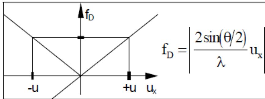
Figure 4-3 Directional ambiguity without frequency shift. [11]
