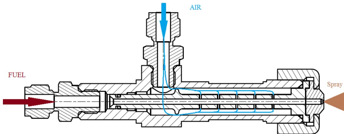
Figure 3-2 Principle of the construction.
