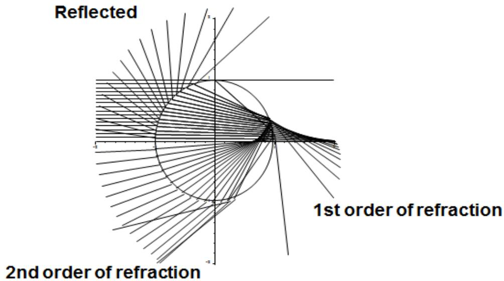
Figure 4-13 Scattering modes (water bubble in air). [12]
