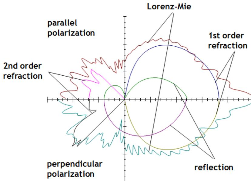
Figure 4-5 Lorenz-Mie scattering theory (the light intensity is shown on a logarithmic scale). [11]
