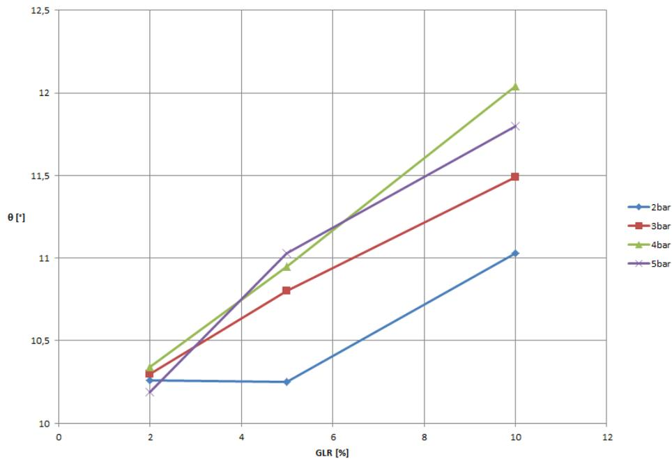
Figure 7-6 Cone angle at 21°C.
