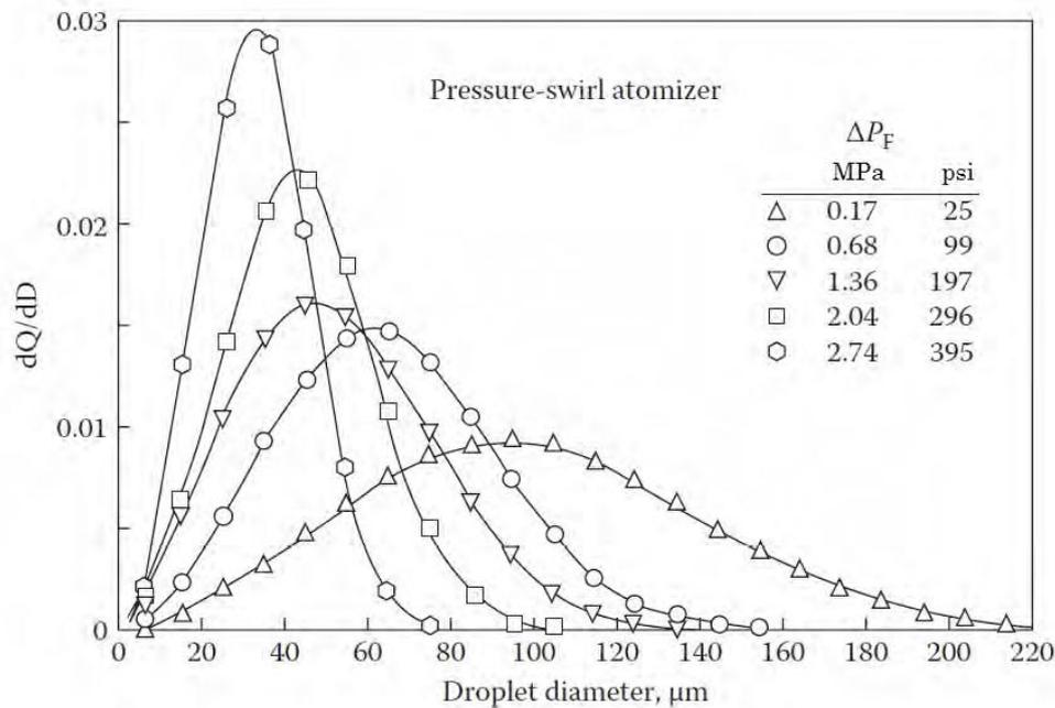
Figure 2-12 Dependence of pressure on the droplet diameter. [1]
