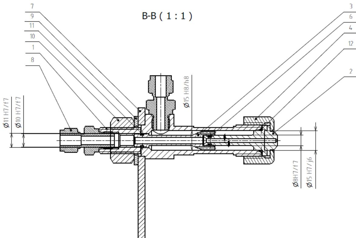
Figure 3-3 Construction for "short" atomizers with reduction part.
