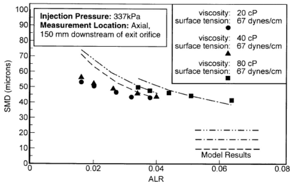
Figure 2-10 Dependency between viscosity on SMD. [5]
