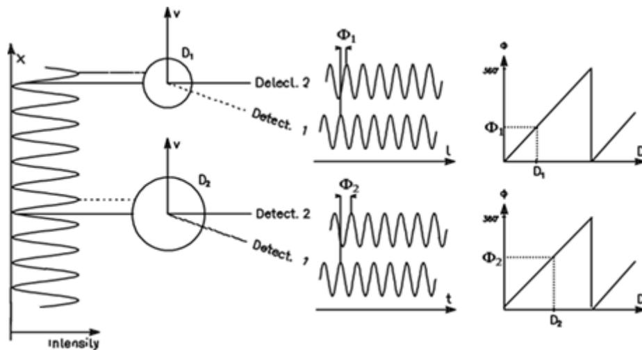
Figure 4-14 Phase difference in relationship to particle diameter. [11]
