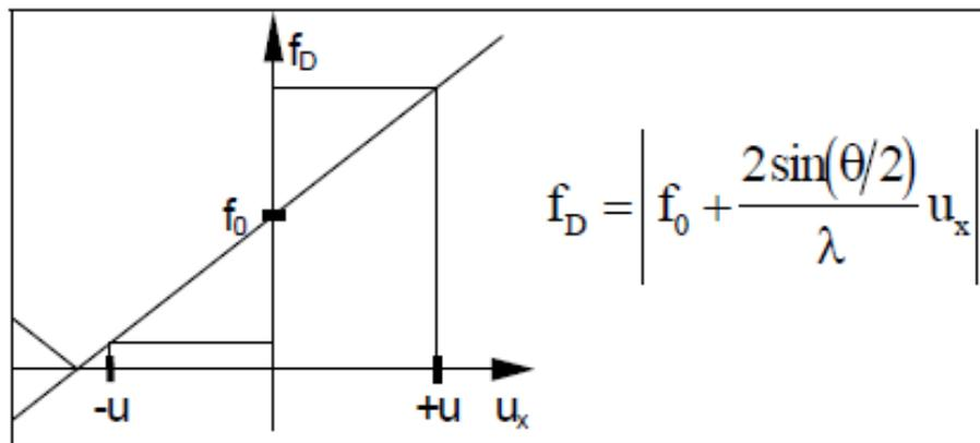
Figure 4-4 Directional ambiguity using frequency shift. [11]
