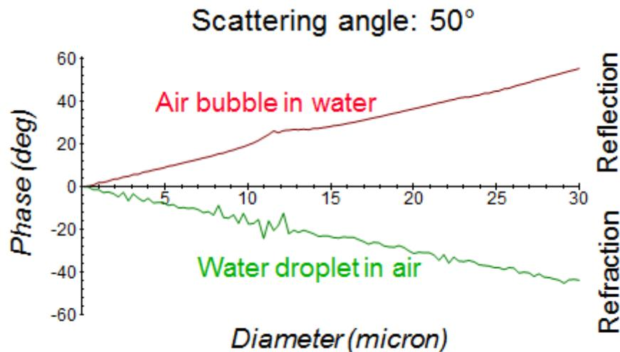
Figure 4-11 Phase-diameter linearity. [12]
