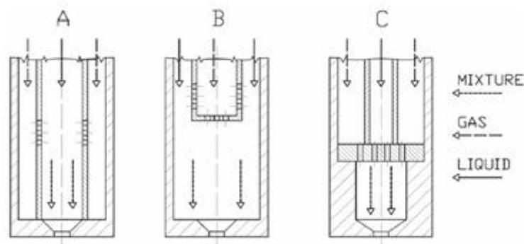
Figure 2-3 Different constructions of effervescent atomizers. [6]
