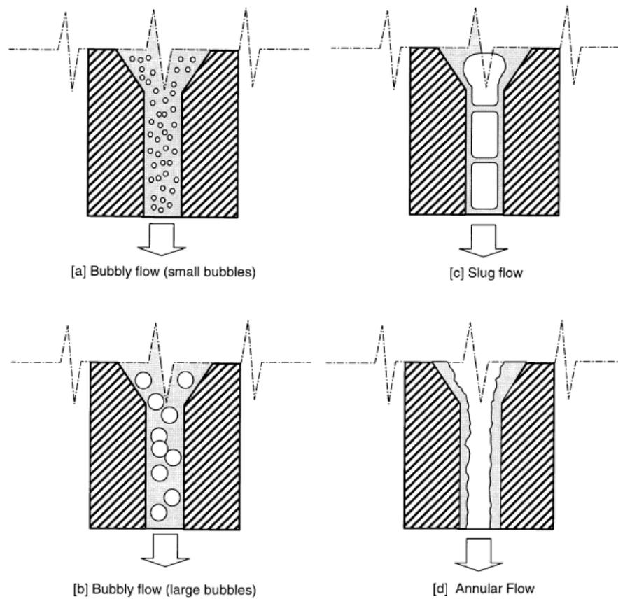
Figure 2-5 Different flow regimes in the discharge orifice. [5]
