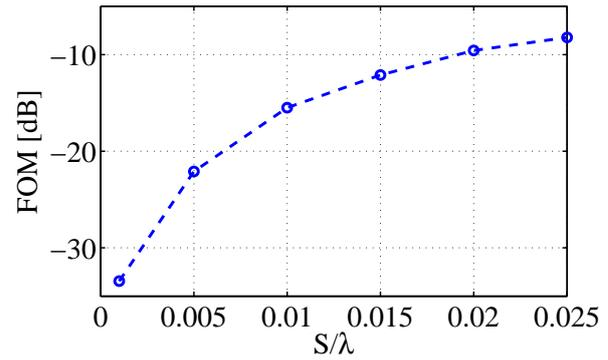
**Fig. 4.** Figure of merit to calculate the deviations between the presented equations and the FIT for different feeding width.  $L = 225$  mm,  $W = 20$  mm, operating frequency = 300 MHz.
