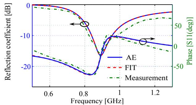
**Fig. 5.** Simulated and measured reflection coefficients as a function of frequency.
