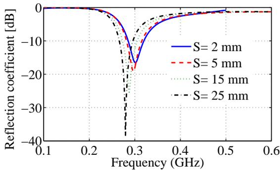
**Fig. 3.** Reflection coefficients as a function of frequency for different feeding width  $S$ .  $L = 225$  mm,  $W = 20$  mm, operating frequency = 300 MHz.
