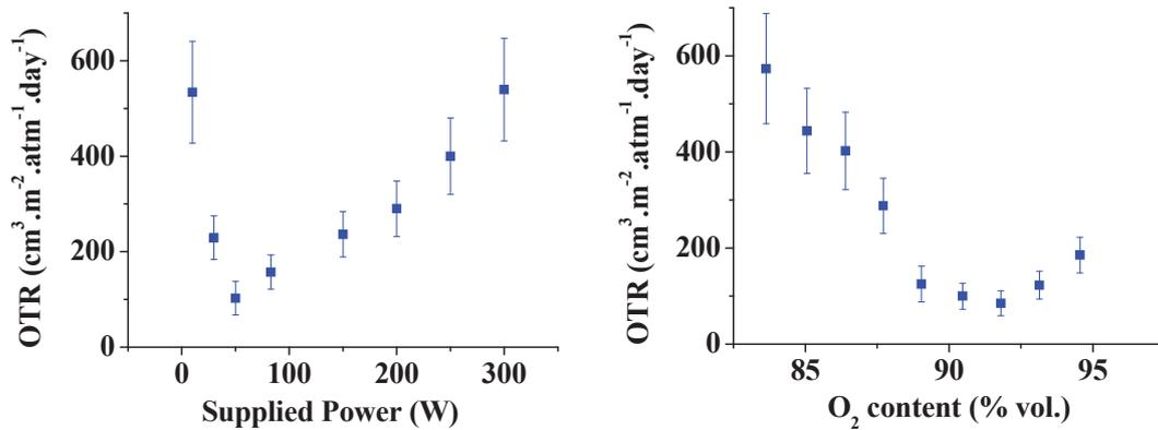
**Figure 2.** Dependence of oxygen transmission rate on supplied power (left) and O<sub>2</sub> content in reaction mixture (HMDSO+O<sub>2</sub>) (right).
