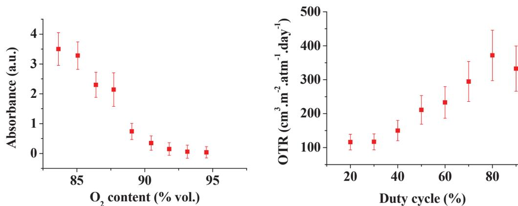
**Figure 3.** Dependence of IR absorbance of Si-(CH<sub>3</sub>)<sub>x</sub> on O<sub>2</sub> content in reaction mixture (HMDSO+O<sub>2</sub>).
