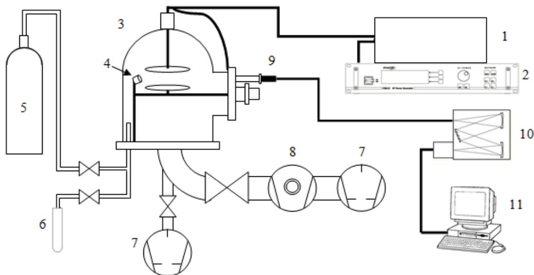
**Figure 1.** Apparatus for PECVD with HMDSO precursor.
