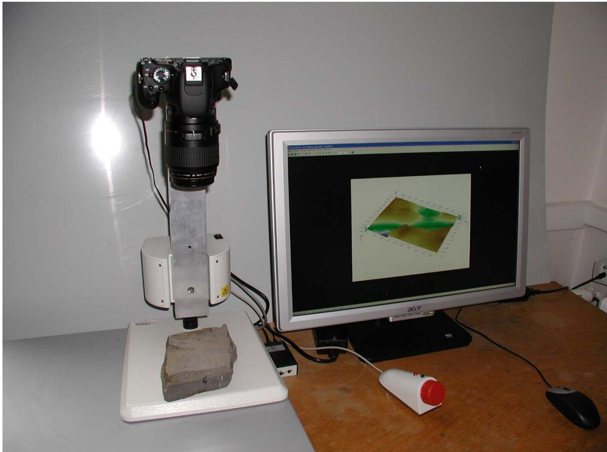
**Figure 1.** Digitizing device used for laboratory reconstructions of 3D reliefs of rock joints
