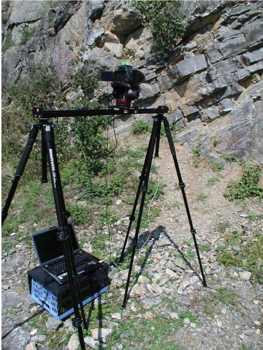
**Figure 2.** Digitizing device used for terrain reconstructions of 3D reliefs
