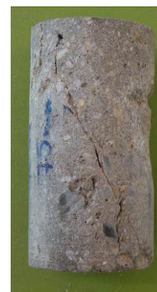
Figure 5. Sample after triaxial test at \sigma_1 = -8 MPa with diagonal shear crack.
