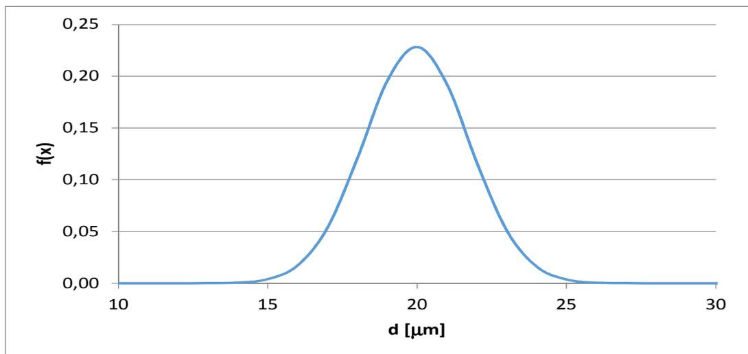
**Figure 2.** Diagram of the normal distribution of the fiber thickness in the PES sample (probability density).
