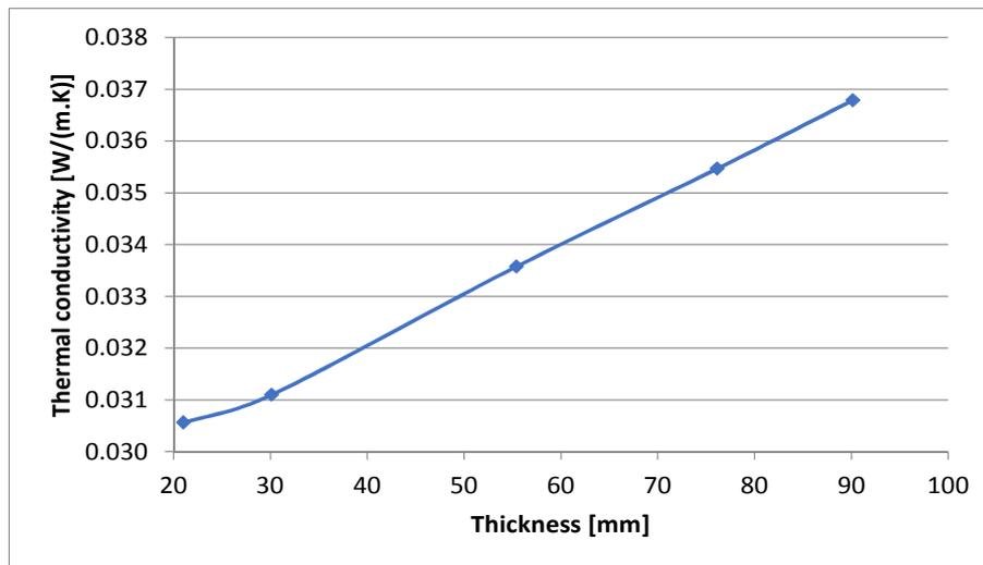
**Figure 5.** Diagram showing the dependence of thermal conductivity on thickness.
