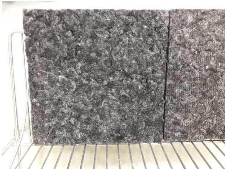
**Figure 3.** Photograph of a specimen with density of 100 kg/m<sup>3</sup>.
