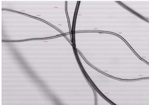
**Figure 1.** Microscopic image of the PES fibers.
