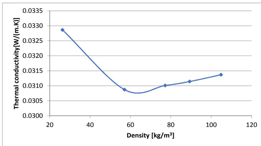
**Figure 4.** Diagram showing the dependence of thermal conductivity on bulk density.
