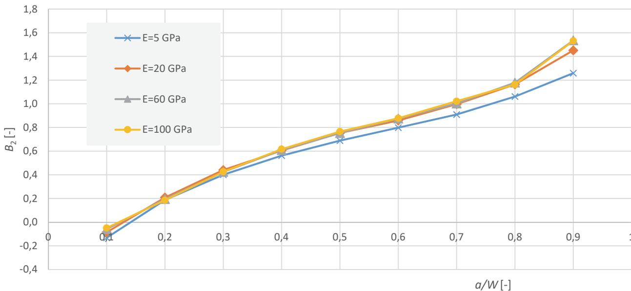
Figure 5: Values of dimensionless  $B_2$  factor ( $T$ -stress) versus  $a/W$ , the effect of elasticity modulus ratio (steel  $E=210$  GPa).
