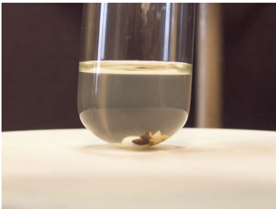
Figure 21 Detail of carbene generation reaction after 40 minutes activation period.
