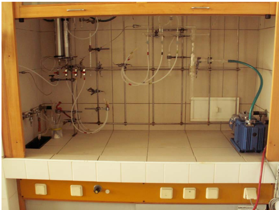
Figure 19 Vacuum line- manifold for experiments under inert atmosphere at Polymer Synthesis Laboratory at Faculty of chemistry BUT.
