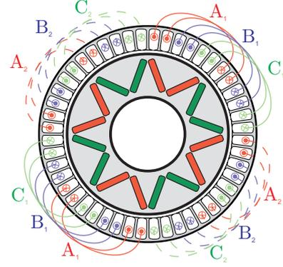
Fig. 3. Double three-phase motor with distributed winding and segregated sub-systems.
