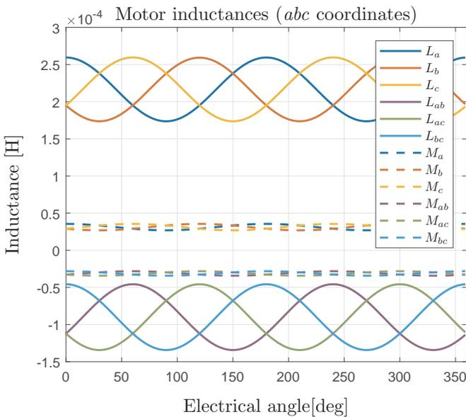
Fig. 4. Inductances of analysed double three-phase motor with low mutual inductances between sub-systems.
