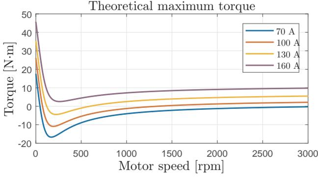
Fig. 8. Theoretical maximum motor torque (one sub-system active and second sub-system in ASC).
