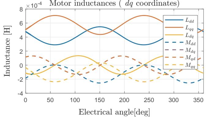
Fig. 10. Inductances of double three-phase motor with segregated sub-systems transformed into  $dq$  coordinates.
