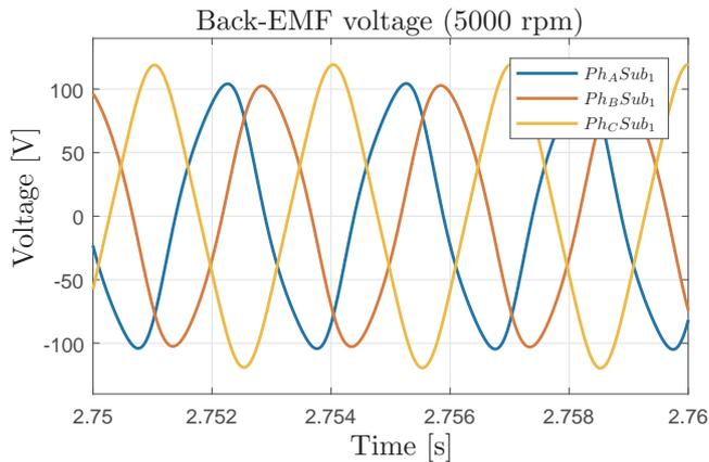
Fig. 11. Back-EMF phase voltage of double three-phase motor with phase shift between sub-systems.
