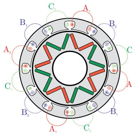
Fig. 1. Double three-phase motor with non-overlapping concentrated winding and interlaced sub-systems.
