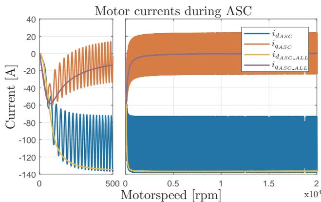
Fig. 12.  $dq$  currents of ASC sub-system.
