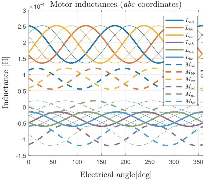
Fig. 6. Inductances of double three-phase motor with high mutual inductances between sub-systems.
