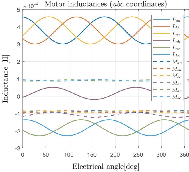
Fig. 9. Inductances of double three-phase motor with segregated sub-systems
