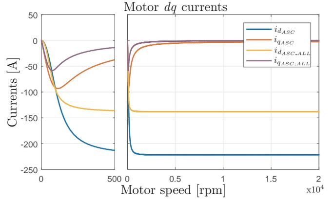
Fig. 7. Motor currents during ASC in both sub-systems
