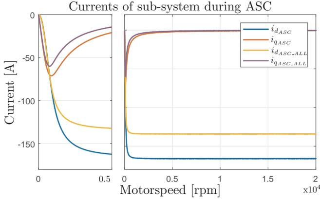
Fig. 5.  $dq$  currents of ASC sub-system.
