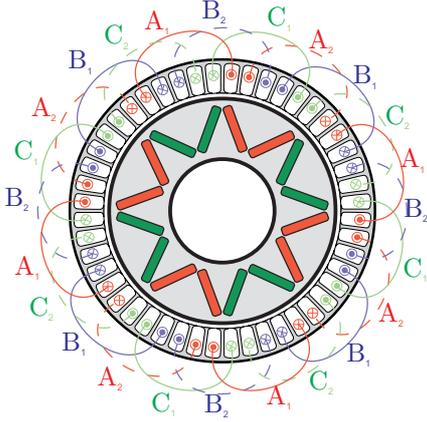
Fig. 2. Double three-phase motor with distributed winding and interlaced sub-systems.
