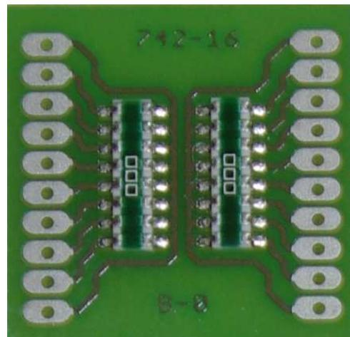
**Figure 2:** (a) Temperature profile for soldering by vapors (b) Assembled test board with soldered resistor arrays
