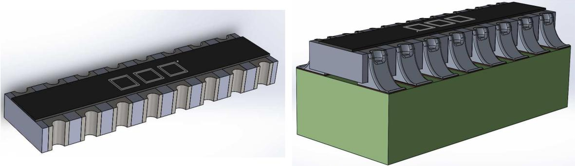
**Figure 3:** Solidworks – (a) model of ceramic resistor array (b) complete model of ceramic resistor array with FR-4 substrate
