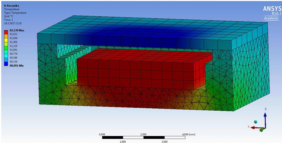
**Figure 5:** Temperature distribution with 120mW power load.
