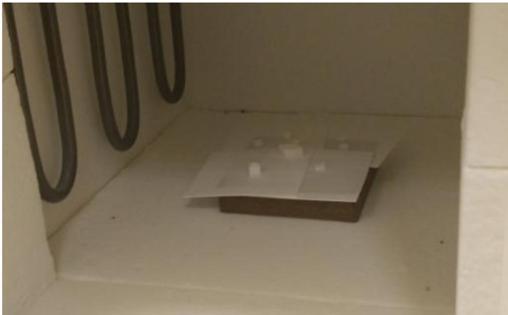
**Figure 4:** Chamber of furnace after sintering
