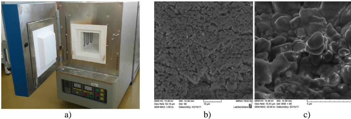
**Figure 3:** a) Furnace ST 1700MX, b) unsintered corundum powder, c) sintered corundum powder
