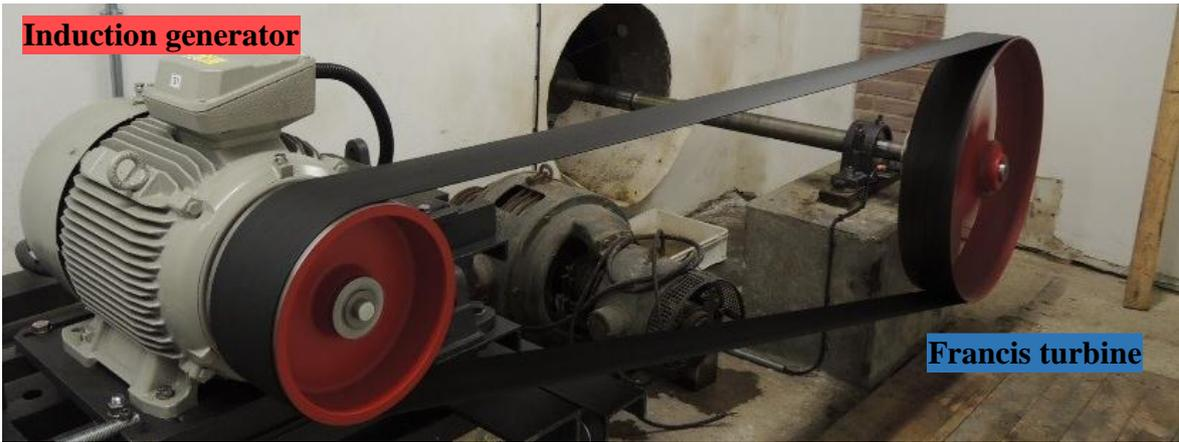
**Figure 1** View on the generator and output shaft of the small hydro power plant
