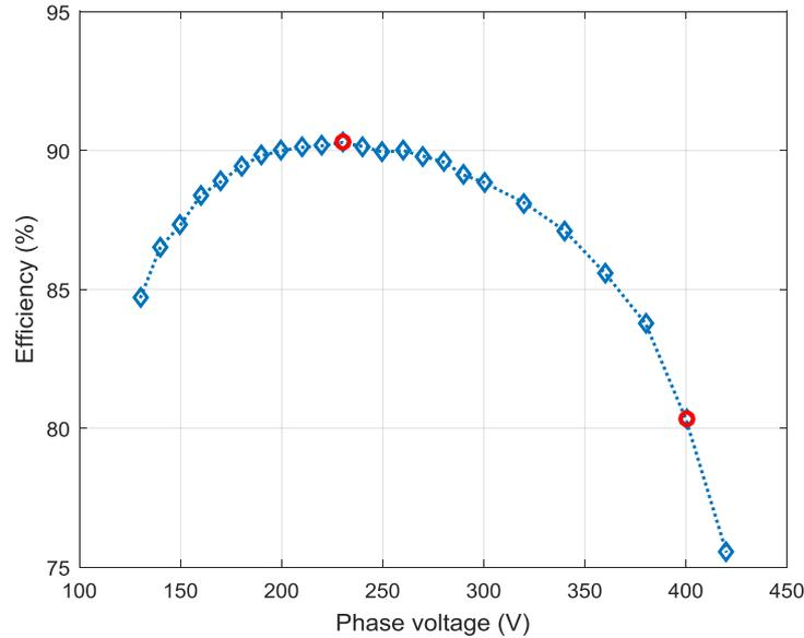
**Figure 5** Efficiency of the generator in dependence on the stator voltage [4]
