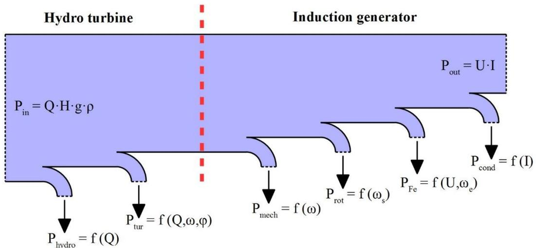
**Figure 3** Power losses in a hydro power plant
