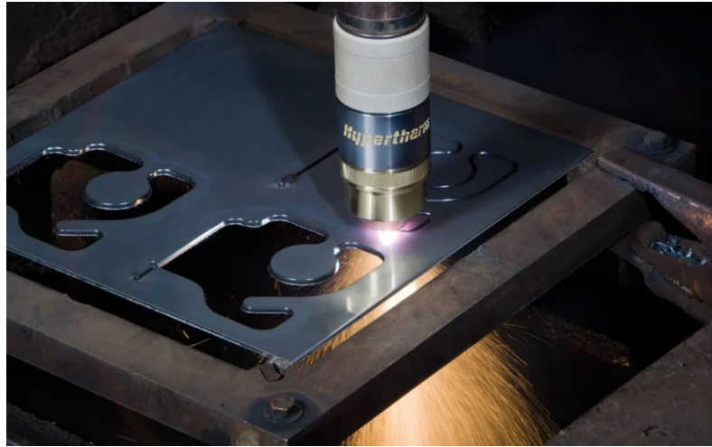
Figure 2.3: Plasma cutter in operation [1]
