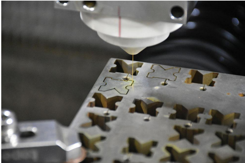
Figure 2.5: Wire EDM cutting a thick piece of material [26]
