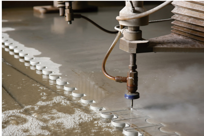
Figure 2.4: Detail of a waterjet cutting stainless steel [35]
