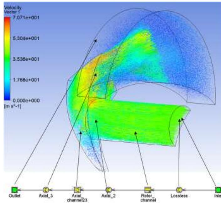
Fig. 2. Axial intake port 3D calibration
