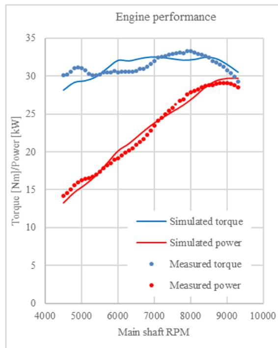
Fig. 3. Engine prediction correlation with measured data
