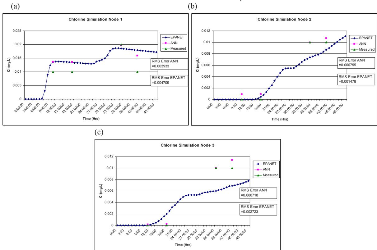
Fig. 5. ANN and EPANET Simulation in (a) node 1; (b) node 2; and (c) node3
