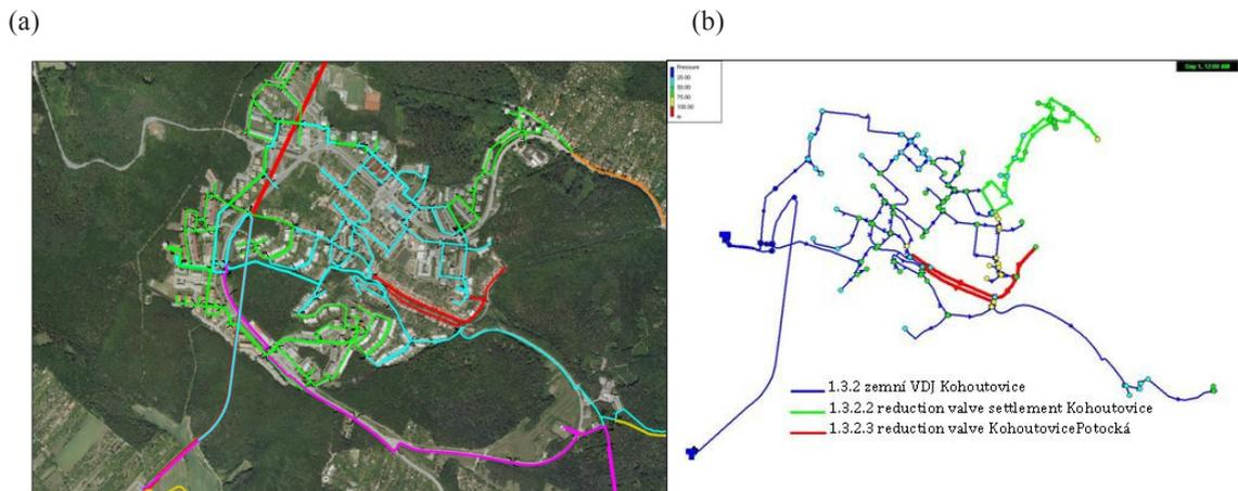
Fig. 2. (a) Water supply scheme, (b) Hydraulic model run in EPANET 2.0
