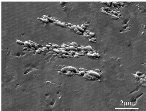
Fig. 1. Surface slip markings on UFG Cu, gigacycle fatigue  $5 \times 10^9$  cycles
