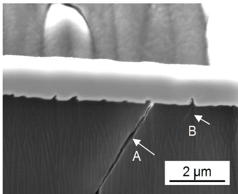
Fig.3. Profile of slip markings and fatigue cracks in UFG AZ91.
