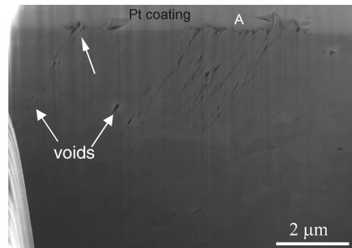
Fig. 2. Profile of slip markings on UFG Cu and subsurface damage, gigacycle fatigue
