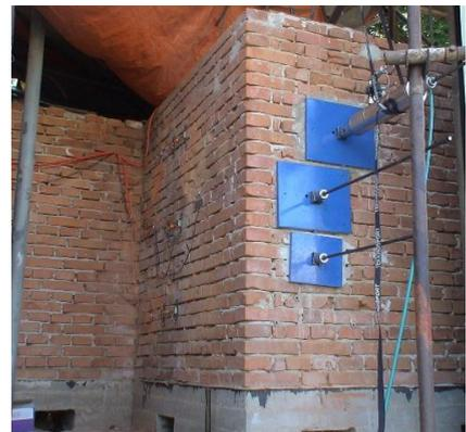
Fig. 2. (a) Plan of vertical prestressing; (b) View of measured model (three brick walls)
