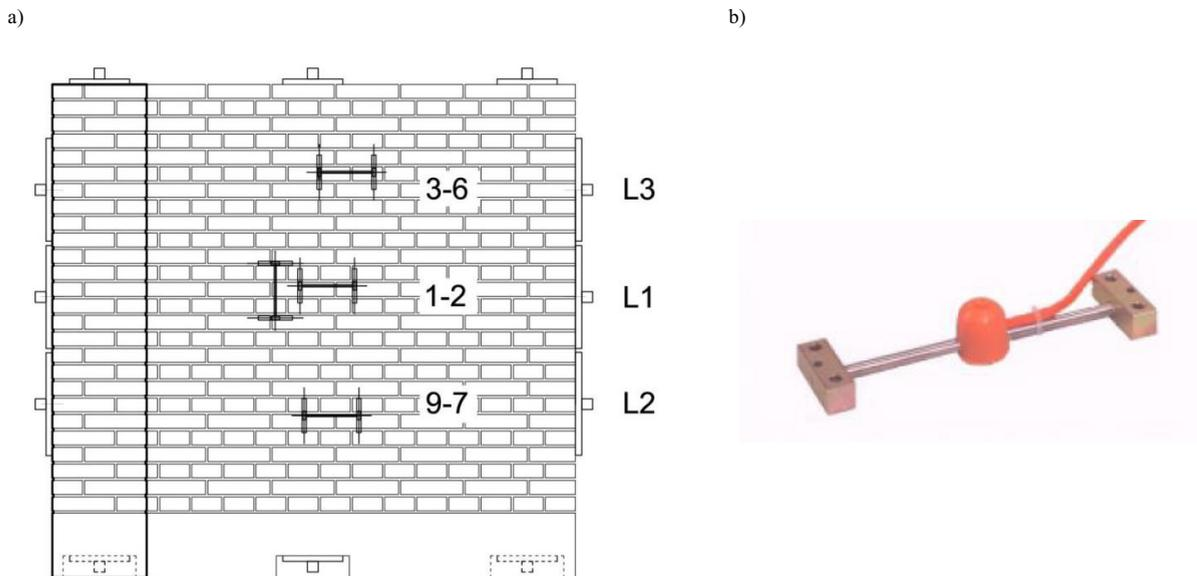
Fig. 3. (a) Labelling of strain gauges; (b) Wire strain gauges
