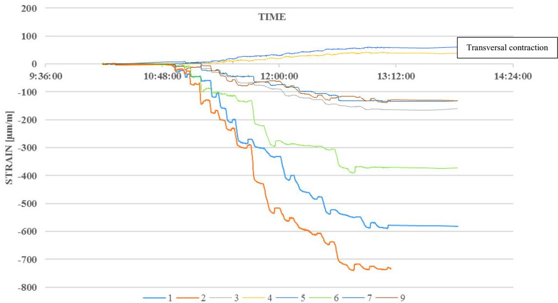
Fig. 6. Short-term monitoring of deformation during prestressing of horizontal cables. Gauges no. 4 and 5 have been shown transversal contraction
