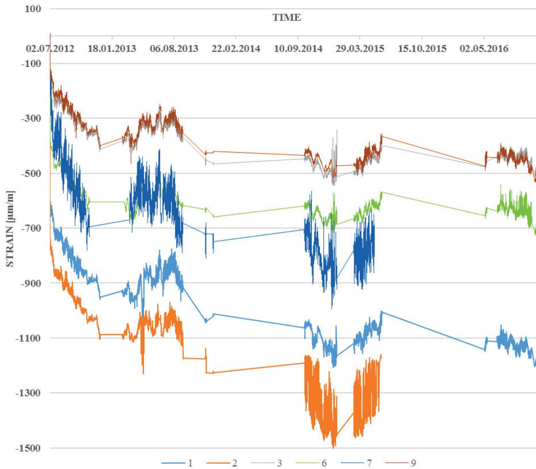
Fig. 4. Long-term monitoring of deformation [ $\mu\text{m/m}$ ]. In the middle section is strain highest (gauges no. 1 and 2)
