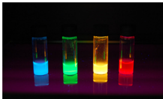
Fig. 1 Picture shows synthetic blue, green, yellow and red QDs respectively after illumination using UV transilluminator (254 nm). (Color figure online)
