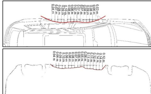
Figure 10: Skoda Kodiaq side impact – top-view (up) vs. scanner (down).
