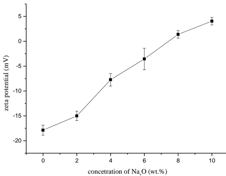
*Fig. 25: Dependence of the zeta potential ( $\zeta$ ) on the wt.% of  $\text{Na}_2\text{O}$  in NaOH activator*
