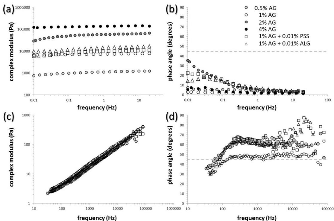
**Figure 1.** Parameters of viscoelasticity of the gels determined on macroscopic (a,b) and microscopic scale (c,d). Frequency dependence of the complex modulus (a,c) and the phase angle (b,d), respectively.
