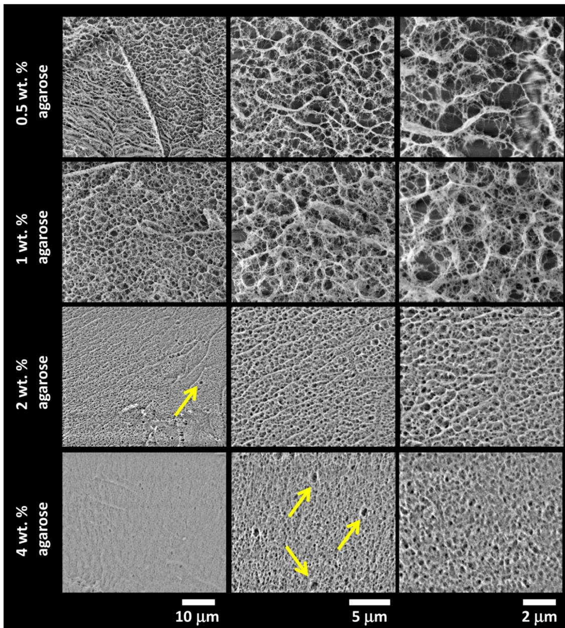
**Figure 4.** Results of cryogenic scanning electron microscopy (cryo-SEM) imaging of the internal structure of the plunge-frozen hydrogels with various content of agarose (with the absence of an interpenetrating polyelectrolyte component). Structure alterations caused by the formation of ice crystals are marked with arrows.
