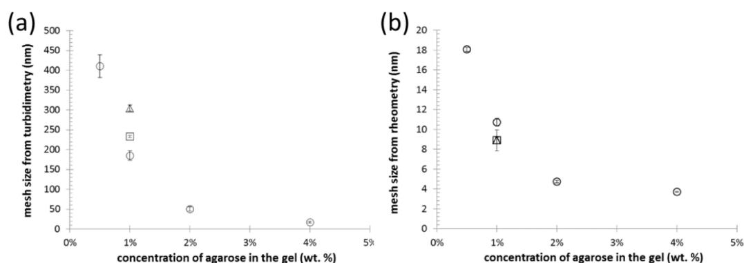
**Figure 3.** Results of indirect structural mapping of the hydrogels with different concentrations of agarose (○) and of the gels containing 1 wt.% of agarose-based interpenetrated by 0.01 wt.% of PSS (□) and ALG (Δ), respectively. The analysis-specific effective mesh sizes were calculated from the results of turbidimetry (a) and (macro)rheometry (b), respectively.
