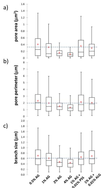
**Figure 7.** Box plots of pore size parameters determined from analysis of cryo-SEM images using ImageJ software. (a,b) Pore areas and perimeters determined using the ‘Analyze Particles’ tool. (c) Branch sizes using the ‘Analyze skeleton’ tool. Blue dashed lines in the box plots represent the mean values of the displayed parameters for 1 wt.% agarose gels without the presence of an interpenetrating polyelectrolyte component.
