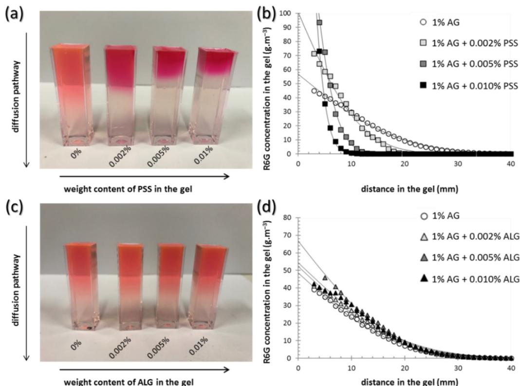
**Figure 2.** Diffusion of Rhodamine 6G (R6G) in the gels investigated on the macroscopic scale. (a,c) Visual comparison of agarose gels (1 wt.% of agarose) with different content of the interpenetrating component after 72 h of diffusion of R6G from solution. (b,d) Experimentally determined concentration profiles of the same gels.
