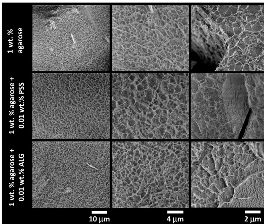
**Figure 5.** Results of cryo-SEM imaging of the internal structure of the plunge-frozen 1wt.% agarose hydrogels with and without the presence of an interpenetrating polyelectrolyte component (0.01 wt.% of PSS and ALG, respectively).
