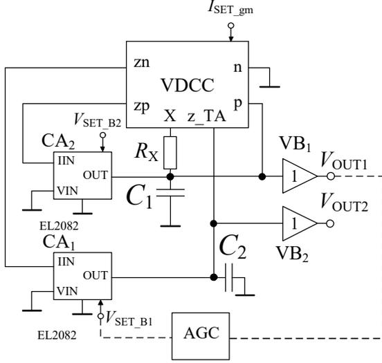
Fig. 1. Circuit diagram of the proposed oscillator.
