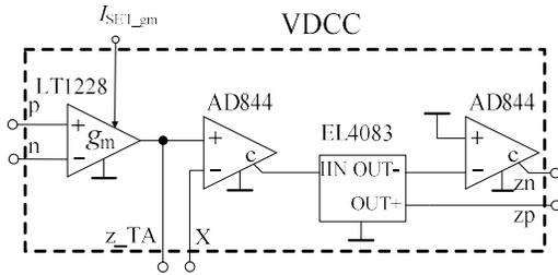
Fig. 2. CG-VDCC element realization using commercially available devices
