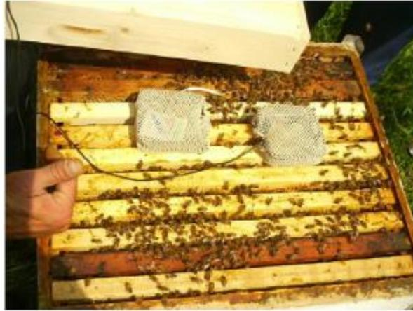
**Figure 2:** Placement of the microphone and the data logger in the bee hive [6]
