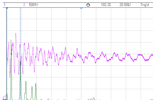
Figure 2: Mechanical response of 4-layer piezoelectric actuator
