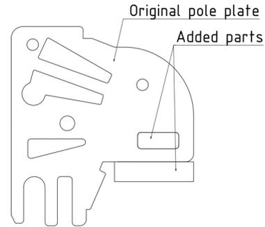
**Figure 4:** Pole plate alterations
