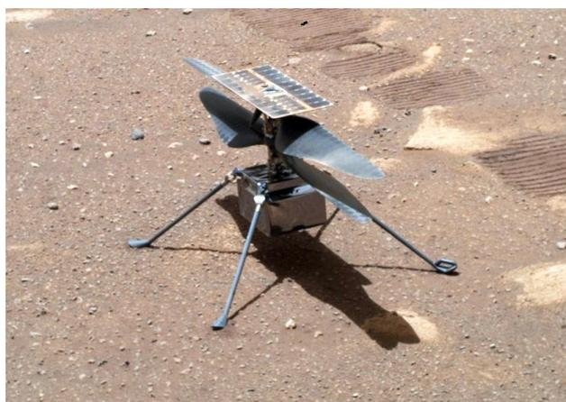
**Figure 8.** Image of the Ingenuity helicopter on Mars acquired on 7 April 2021 (Sol 46). IMM multi-junction solar cells are clearly visible from its top [64].
