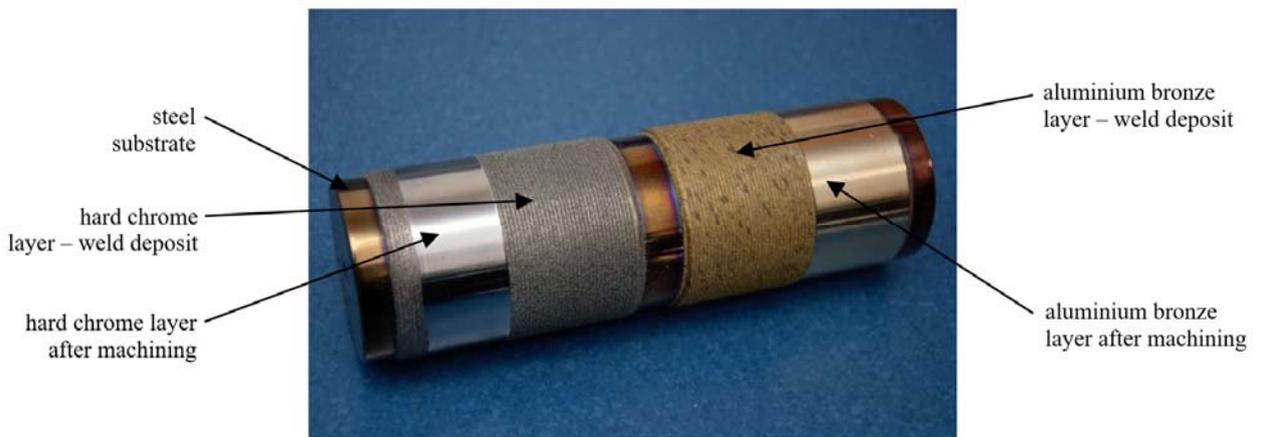
Fig. 3. Real specimens of a steel cylinder coated with a hard chrome layer and/or an aluminium bronze layer.
