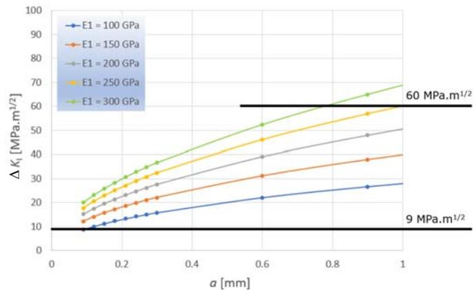
Fig. 7. Dependence of the stress intensity factor range on the crack length for various Young's moduli of the cladded layer with the thickness  $h_1 = 3$  mm.
