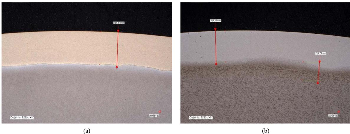
Fig. 1. 50× zoomed steel core with (a) aluminium bronze layer; (b) hard chrome layer.
