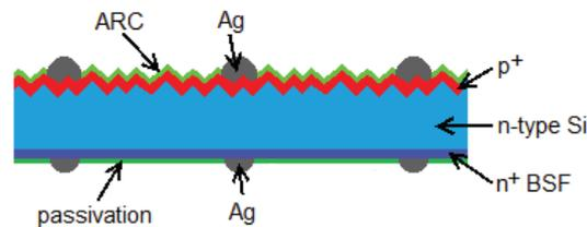
Fig. 1. schematic cross-section of the investigated  $n$ -PERT cells.
