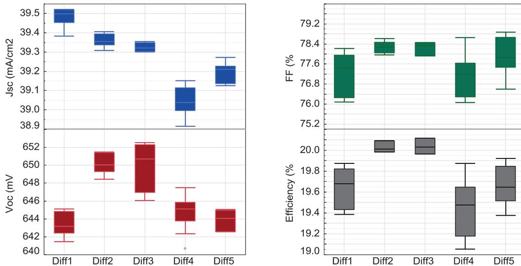
Fig. 4. solar cell parameters obtained by IV measurement at 25 °C and under AM1.5 spectrum with illumination intensity of 1000 W/m<sup>2</sup>.
