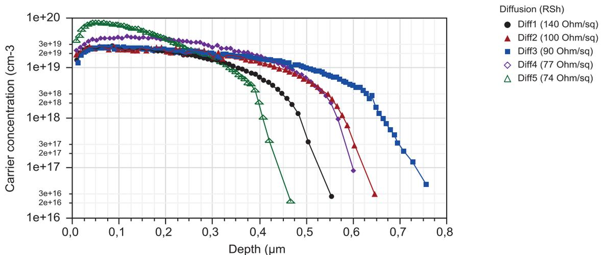
Fig. 2. ECV profiles of the investigated boron diffusion.
