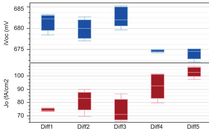
Fig. 3.  $iV_{OC}$  at 1 sun and  $J_0$  of the cell precursors (before metallization). The  $J_0$  was extracted at an injection level of  $\Delta n = 3 \times 10^{15} \text{ cm}^{-3}$ .
