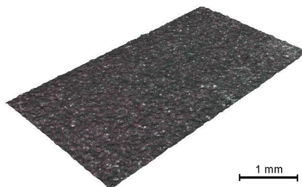
FIGURE 8. Non-filtered image of the surface of sample 30,  $2.5 \times$  magnified (voltage 70 V,  $T_{\text{on}} = 6 \mu\text{s}$ ,  $T_{\text{off}} = 30 \mu\text{s}$ , wire feed 14 m/min, current 35 A).
