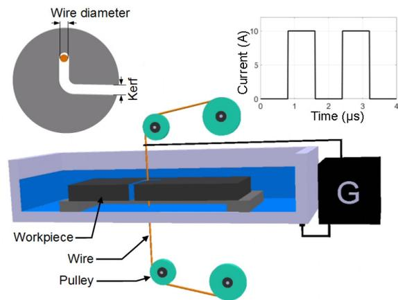
FIGURE 1. Diagram of wire electrical discharge machining process.
