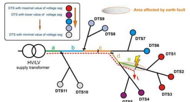
Fig. 3 Operation principle of the method for EF location
