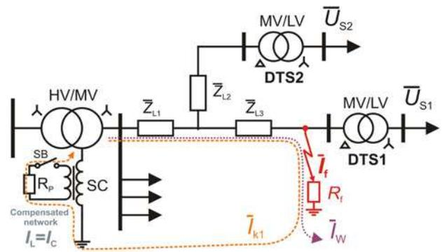
Fig. 1 Way of a residual current through faulty line during EF in compensated network
