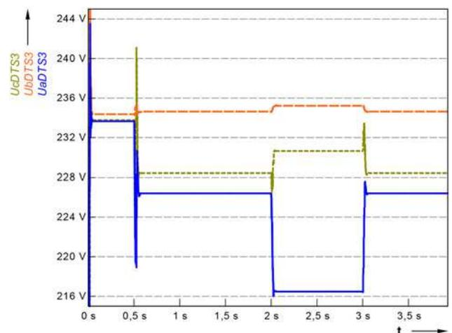
**Fig. 9** RMS phase voltage waveforms on the LV side of DT during EF in phase A for over-compensated state
