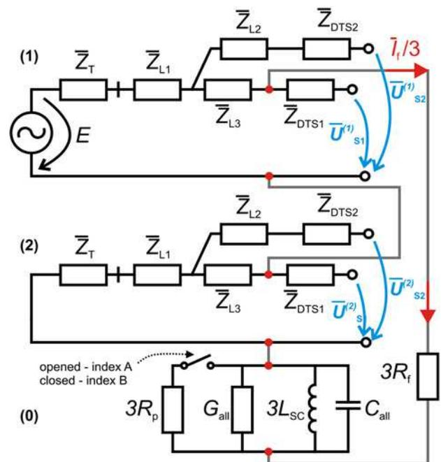
Fig. 2 Symmetrical components scheme of single-phase fault in compensated network
