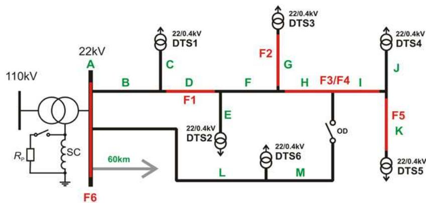
**Fig. 7** Faulty sections delimited by the method during low-impedance EF**Table 2** Recorded maximal voltage sags during  $600 \Omega$  EF at location F1 up to F6
