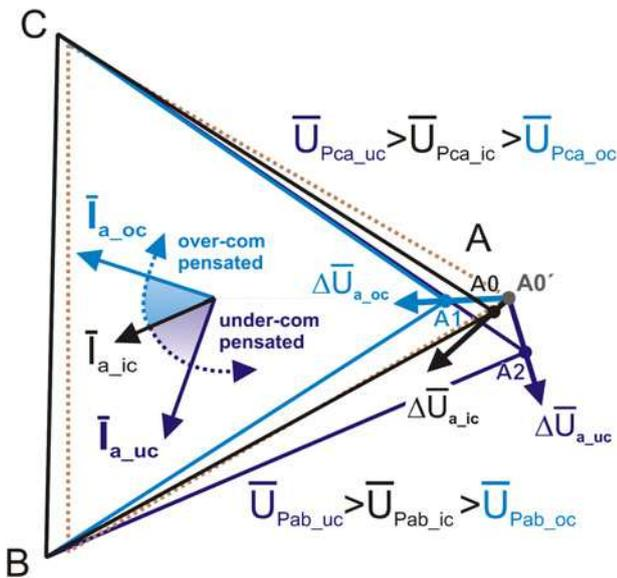
**Fig. 10** Influence of a network compensation state to unbalance of line-to-line voltages in MV system
