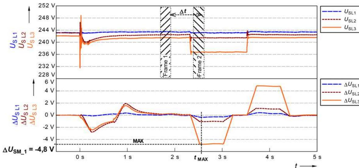
Fig. 4 Example of maximal voltage sag determination for selected DTS during real EF
