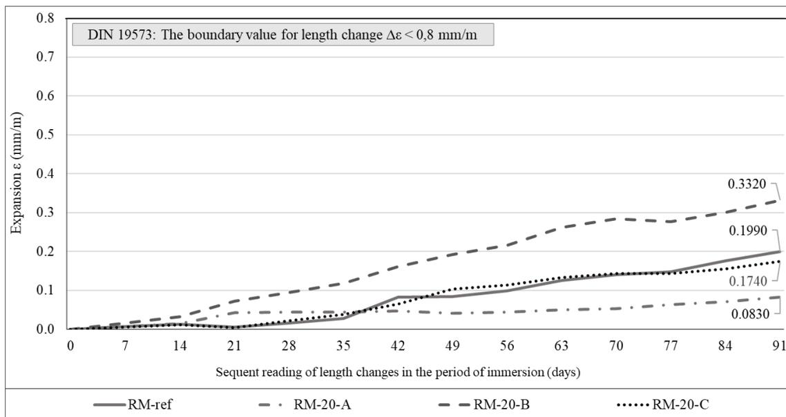
**Figure 1.** Graphical representation of the course of deformation of test specimens exposed to sulphates in time.
