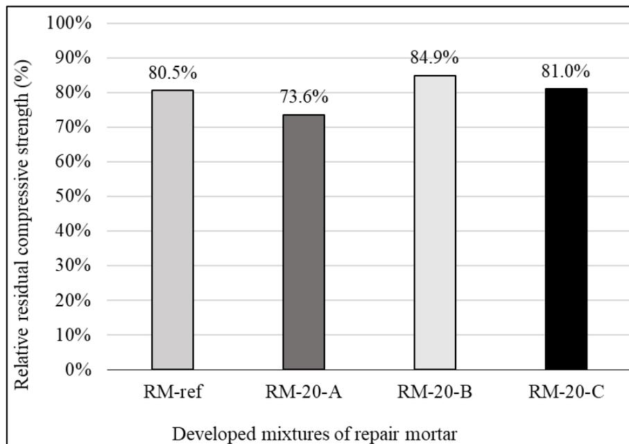
**Figure 2.** Graphical representation of the relative residual compressive strength of the corroded mortar test samples after exposed to a chemically aggressive solution of sulfuric acid ( $H_2SO_4$ ) with a concentration of  $pH = 0$  ( $c(H_2SO_4) = 1.0 \text{ mol/l}$ ) for 14 days.
