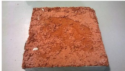
Fig. 2. Detail of colored sample - surface after test of resistance to water and defrosting chemicals according to ČSN 73 1326/Z1, after 100 freeze-thaw cycles (author's photo) - mixture B with pigments.
