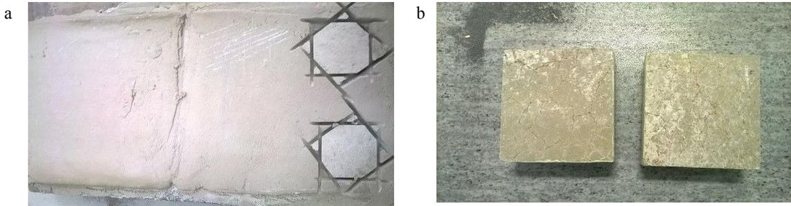
Fig. 1. Details of examined samples (a - author's photo) test of adhesion to the base - mixture B, (b - author's photo) surface after resistance to water and defrosting chemicals to ČSN 73 1326/Z1, after 100 freeze-thaw cycles - mixture C.
