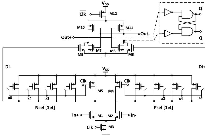
Fig. 6. Improved latch type sense amplifier with offset compensation.
