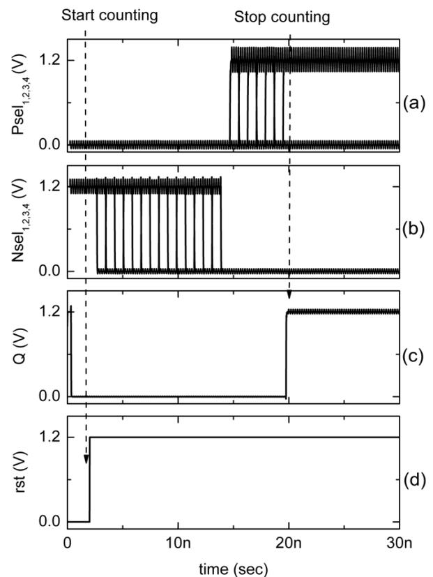
Fig. 7. Counting select bits of a) right side transistors, b) left side transistors and c) reset signal.
