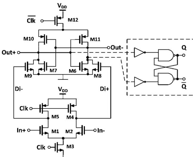
Fig. 3. Improved latch type sense amplifier.
