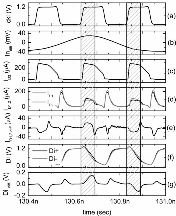
**Fig. 5.** Current and voltage in transistors M1-M5 a) clock b) differential input c) drain current of M3, d) drain current of M1 and M2, e) difference of drain currents of M1 and M2, f) voltage on charging nodes  $D_i$ , g) differential voltage of  $D_i+$ / $D_i-$  nodes.
