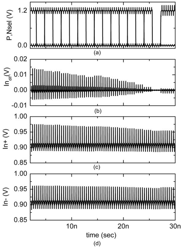
**Fig. 10.** Kickback noise during the offset compensation process a) right side transistors counting, b) kickback on differential input signal, c) kickback on positive input and d) kickback on negative input.
