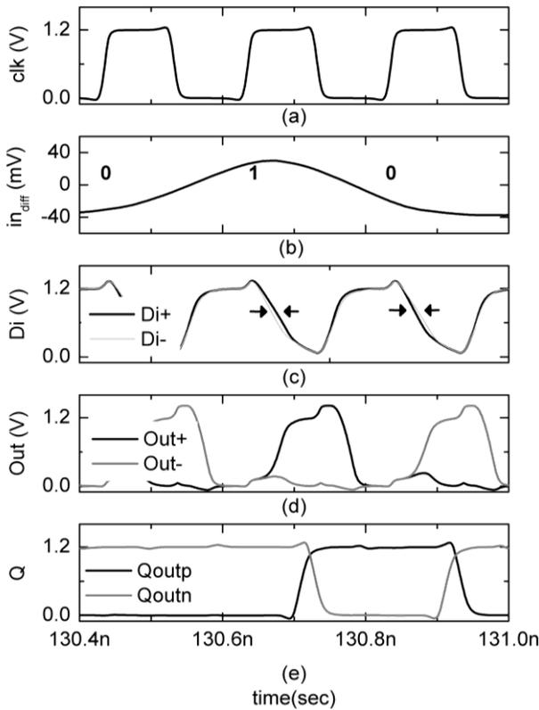
**Fig. 4.** Signaling of the latch type sense amplifier a) clock, b) differential input, c) charging nodes  $Di$ , d) pre-output and e) final output  $Q$ .
