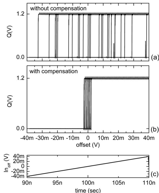
Fig. 8. Offset demonstration a) before and b) after compensation c) with a ramp input signal.
