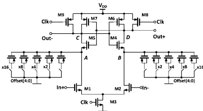
Fig. 2. Offset cancellation scheme based on capacitance control.
