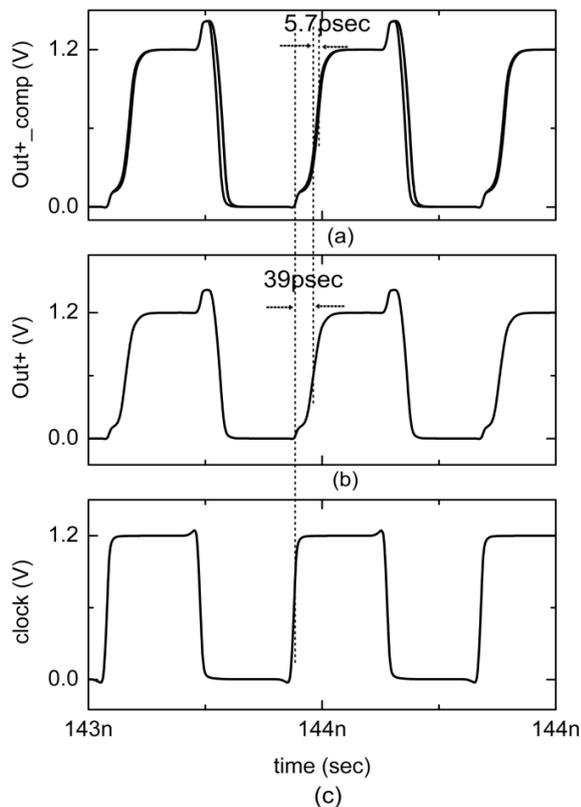
**Fig. 11.** Output delay a) after the offset compensation, b) before the compensation and c) the clock reference.
