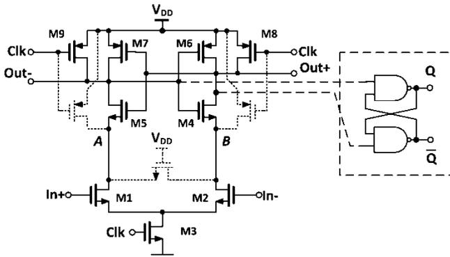
Fig. 1. StrongARM Latch type sense amplifier.
