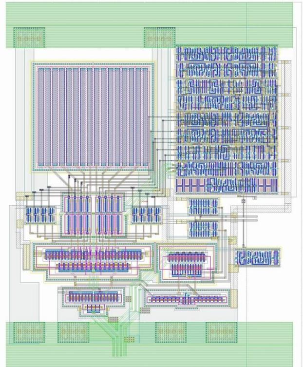
**Fig. 12.** The layout of the latch type sense amplifier.
