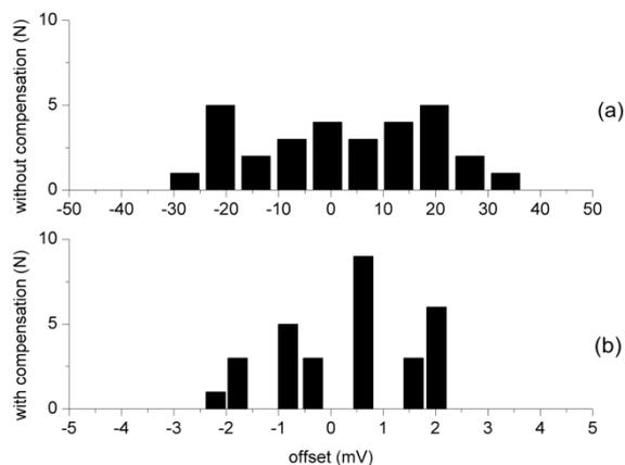
Fig. 9. Offset deviations from Monte-Carlo simulations a) before and b) after compensation.
