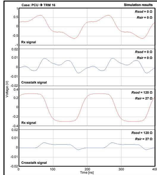
Fig. 5. Effect of serial resistors,  $R_{sod}$  and  $R_{sir}$ , on received and crosstalk voltage level (PCU  $\rightarrow$  TRM 16).
