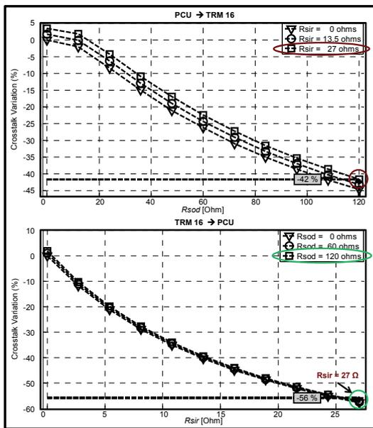
Fig. 7. Effect of serial resistors on crosstalk voltage level.
