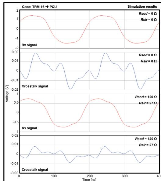
Fig. 6. Effect of serial resistors,  $R_{sod}$  and  $R_{sir}$ , on received and crosstalk voltage level (TRM 16  $\rightarrow$  PCU).
