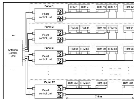
Fig. 1. Interface scheme of SEOSAR/PAZ front end.
