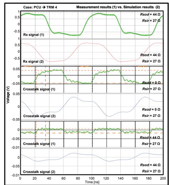
Fig. 9. Comparison of measurement and simulation results (PCU → TRM 4).
