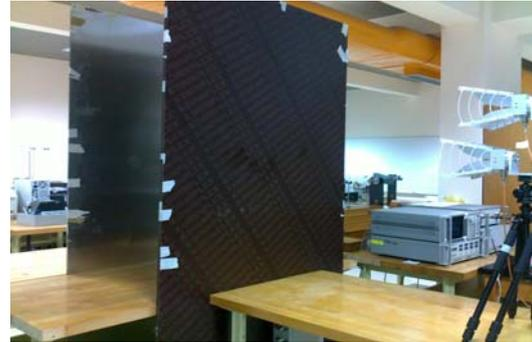
Fig. 2. Through target measurements setup.
