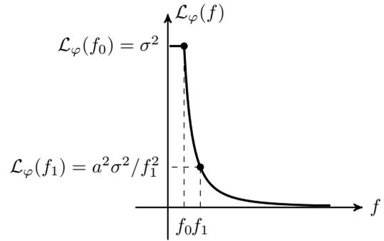
Fig. 7. Model of the carrier phase noise characteristics  $\mathcal{L}_{\varphi}(f)$ .
