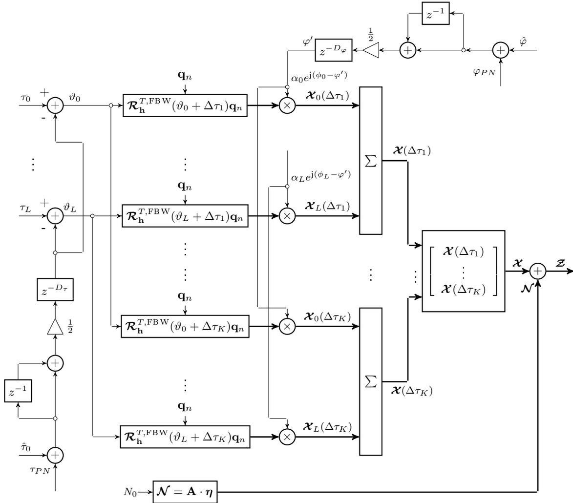
**Fig. 8.** Extended model of the correlator output signals generated as LMDM in slowly fading TDLM in AWGN channel with FBW, feed-back delay, and phase noise. Bold lines represent vectors.
