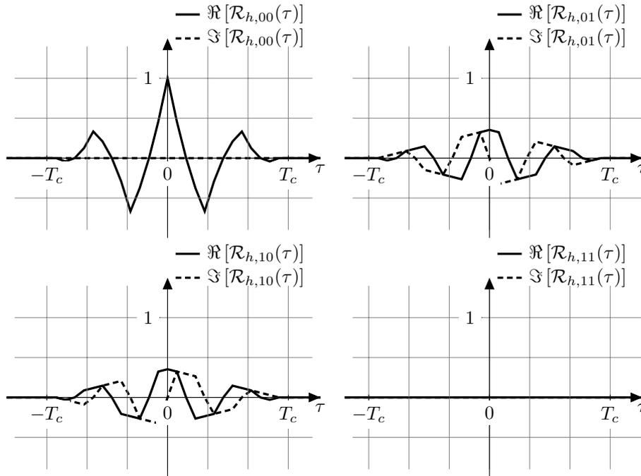
Fig. 4. Correlation functions  $\mathcal{R}_{h,00}, \mathcal{R}_{h,01}, \mathcal{R}_{h,10}, \mathcal{R}_{h,11}$  of the correlation matrix  $\mathcal{R}_h(\tau)$  for LMDM representation of AltBOC(15,10) modulation.
