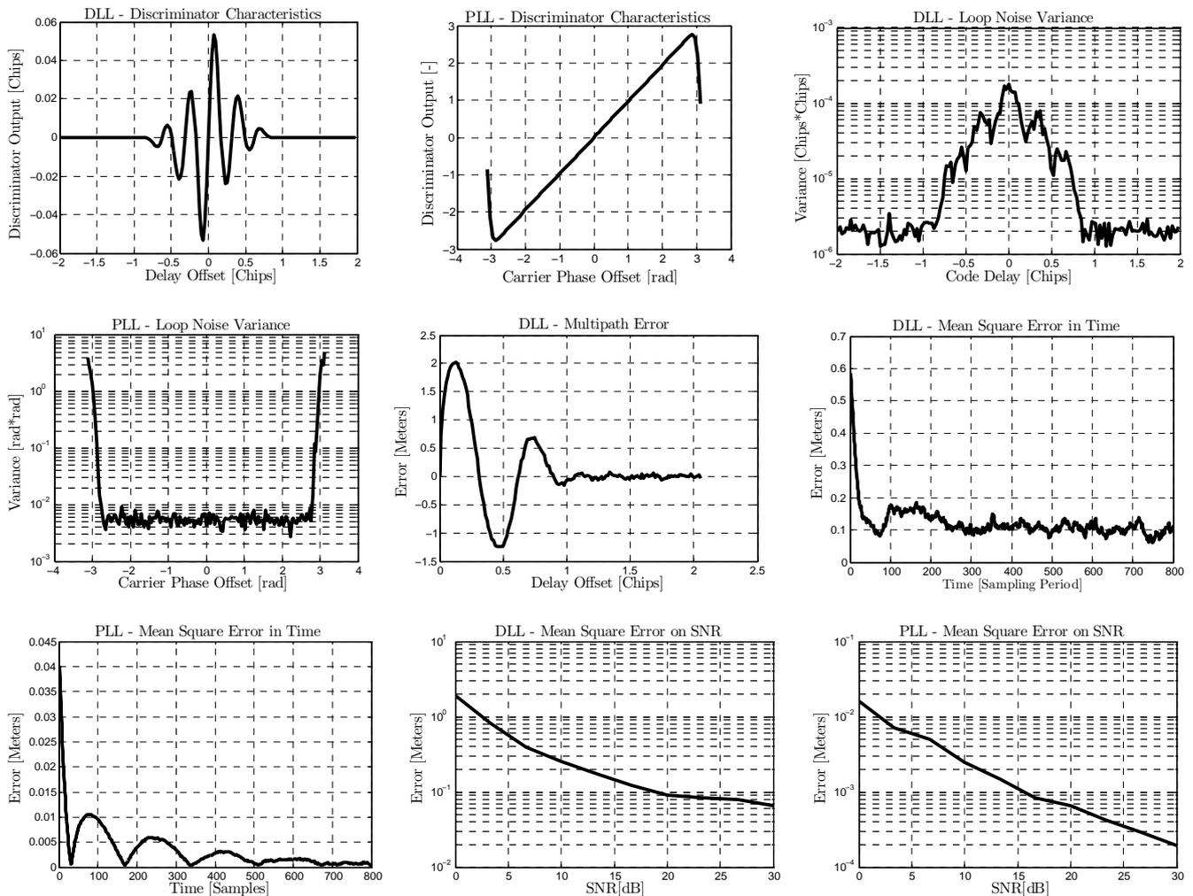
**Fig. 10.** Simulation results of the setup in Tab. 1. The multipath error is evaluated for the difference of carrier phase offsets  $\varphi_1 - \varphi_0 = \pi$  and ratio of amplitudes  $\alpha_0/\alpha_1 = 2$ . The time axes of the mean square error figures are expressed in samples of the post-correlator processing.
