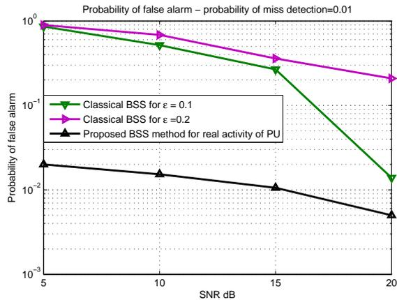
Fig. 9. Probability of false-alarm versus SNR when the probability of miss-detection is constant and equal to 0.01 comparing classical BSS and the BSS using prediction.
