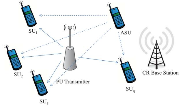
**Fig. 1.** The considered system model in which there are  $q$  SUs, one PU transmitter and one ASU (CR transmitter). Dashed arrows show channels between ASU and other SUs. Plain line arrows show the sensing channel between the PU transmitter and the SUs.
