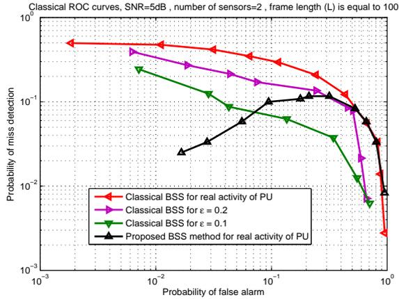
**Fig. 5.** The Classical ROC curve for BSS-based spectrum sensing compared to BSS-based spectrum sensing using prediction unit.
