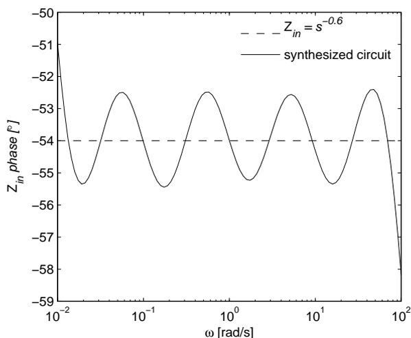
Fig. 10. Comparison of phase of  $Z_{in}$  of the synthesized circuit and the desired function (6).
