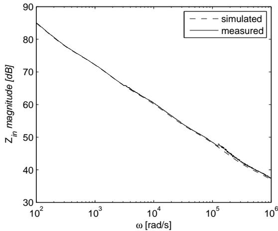
Fig. 15. Comparison of magnitude characteristics for the measurement and the simulation.
