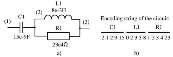
Fig. 1. a) Example of analog circuit, b) its encoding string.
