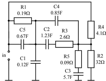
Fig. 7. Schematic of the best found solution.
