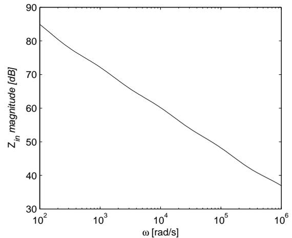
Fig. 13. Magnitude characteristic of  $Z_{in}$  of the transformed circuit.
