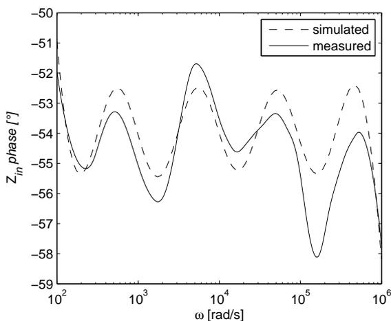
Fig. 17. Comparison of phase characteristics for the measurement and the simulation.
