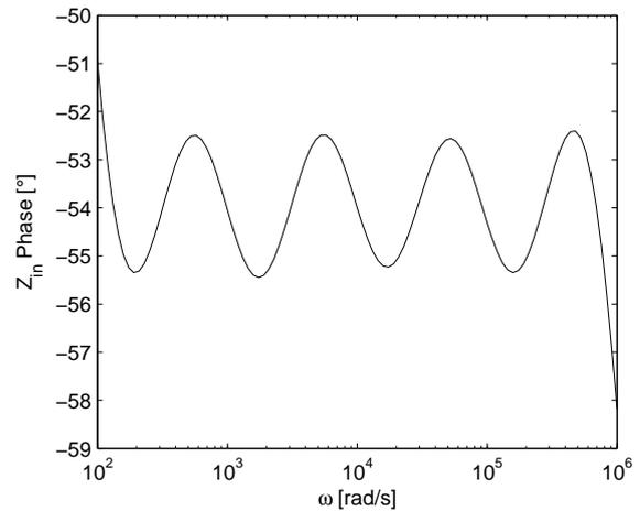
Fig. 14. Phase characteristic of  $Z_{in}$  of the transformed circuit.
