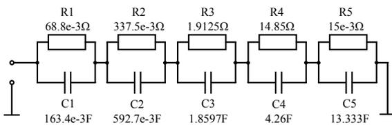
Fig. 2. Schematic of the original approximation circuit.
