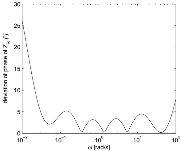
Fig. 6. Phase deviation of  $Z_{in}$  of the original approximation circuit.
