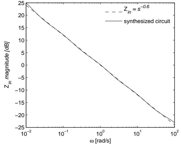
Fig. 8. Comparison of magnitude of  $Z_{in}$  of the synthesized circuit and desired function (6).
