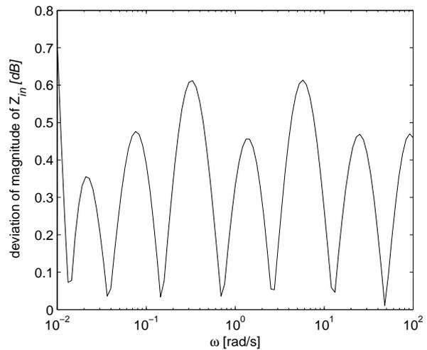
Fig. 4. Deviation of magnitude of  $Z_{in}$  of the original approximation circuit.
