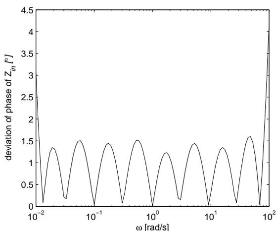
Fig. 11. Phase deviation of  $Z_{in}$  of the synthesized circuit.
