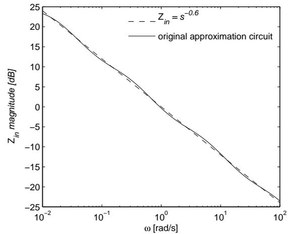
Fig. 3. Comparison of magnitude of  $Z_{in}$  of the original approximation circuit and ideal function (6).
