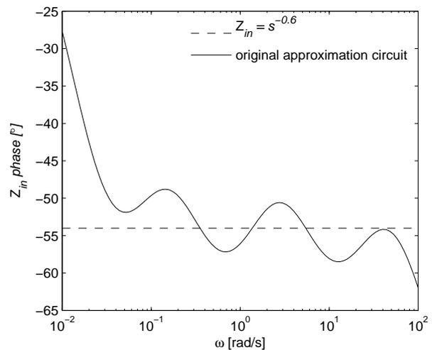
Fig. 5. Comparison of phase of  $Z_{in}$  of the original approximation circuit and ideal function (6).
