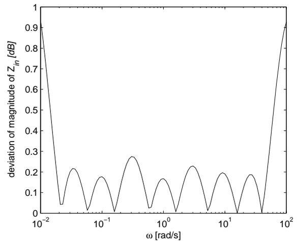
Fig. 9. Magnitude deviation of  $Z_{in}$  of the synthesized circuit.
