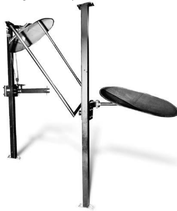
Fig. 5. Mirror system goniophotometer in photometric laboratory of FEI STU
