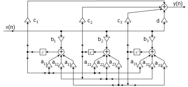
Fig. 6. State-Space filter of the third order in second form.
