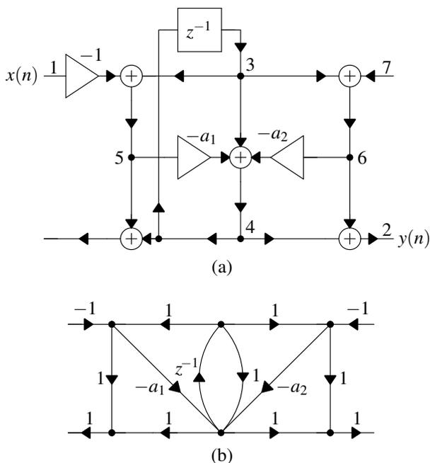
Fig. 2. Parallel adaptor (a) and its signal flow graph (b).
