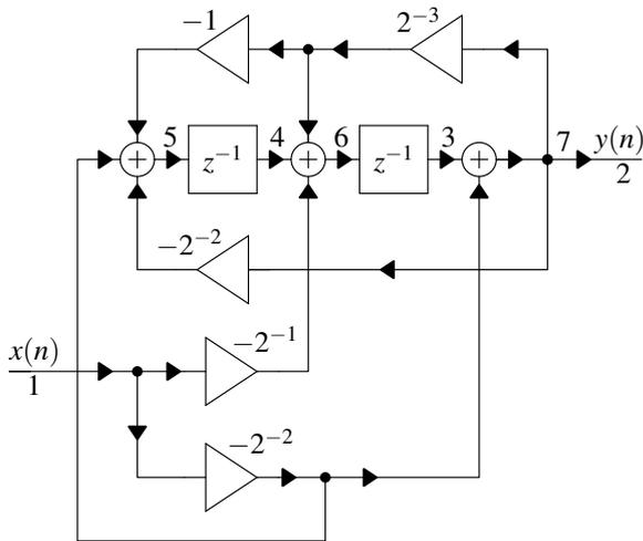
Fig. 4. Filter with four shifting elements and two delay elements.
