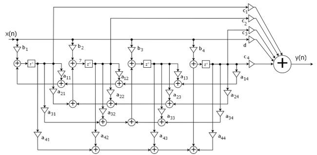
Fig. 7. Direct realization of the State-Space Filter.
