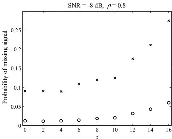
Fig. 3. Probability of missing detection versus  $\tau$ . False alarm probability: x-mark 0.01, circle 0.1.
