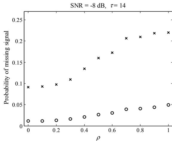
Fig. 4. Probability of missing signal versus  $\rho$ . False alarm probability: x-mark 0.01, circle 0.1.
