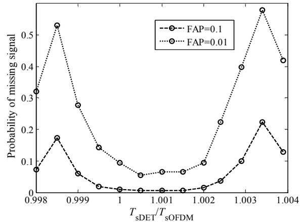
Fig. 7. Dependence of probability of missing signal on sampling interval.
