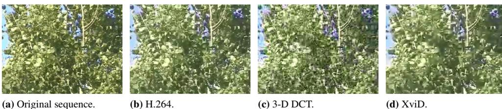
Fig. 8. Sample frames of video sequence Wind encoded by H.264, 3-D DCT and XviD at 500 kbits/s.
