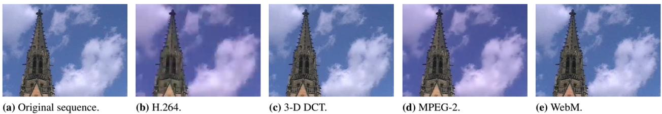
Fig. 5. Sample frames of video sequence Church encoded by H.264, 3-D DCT, MPEG-2 and WebM at 300 kbits/s.
