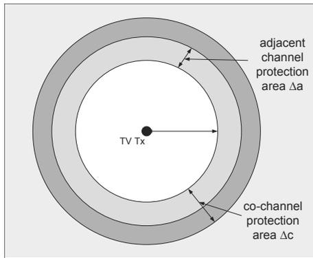
Fig. 1. Considered system model. The TV coverage area is surrounded by secondary users using adjacent channel and co-channel.
